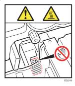
Do not touch the parts a label indicates. The inside of the multi-folding unit could be very hot. Caution should be taken when removing misfed paper.
