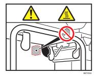
Do not touch the parts a label indicates. The inside of the stacker could be very hot. Caution should be taken when removing misfed paper.
