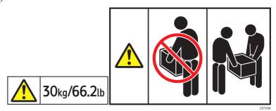
These labels indicate the weight of the unit and describe how to lift the unit. However, these labels are meant for customer engineers. Do not lift a unit that has these labels.
