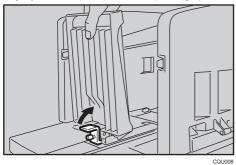
Adjust the angle of the end plate by turning the knob.
