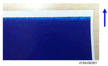
Unprinted area due to insufficient transfer current
