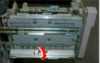
3. Wipe the Paper Exit Inverter Drive Roller [1] with a dry cloth.
