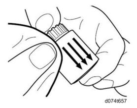
Wipe the entire surface of the paper feed roller lengthwise with a well-wrung-out damp cloth, and then with a dry, unused, lint-free cloth until no moisture remains.
