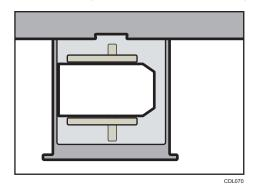
If you are copying onto side-opening envelopes, be sure to unfold their flaps and set them in the  $\Box$  orientation with print side face up. Flaps must be at the right side of the Wide LCT or multi bypass tray (Tray A).
