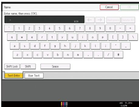
The layout of the keyboard varies depending on the set display language. To use the QWERTY keyboard, press the key displayed on the bottom of the screen, and change the layout of the keyboard. For details about the display language, see page 45 "Changing the Display Language".
