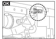
Make sure that the connector and the tube are attached securely.
