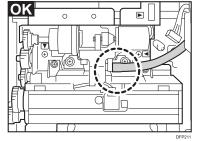
When attaching the connector of the sub-hopper unit, push it to make sure it is inserted fully and squarely.
