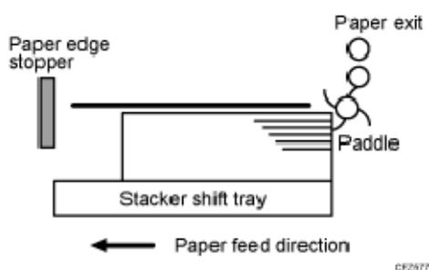
2. Strong friction occurs on the trailing edge so that the paddle cannot pull the sheet back and align the edges of the sheet with those of the stack.
