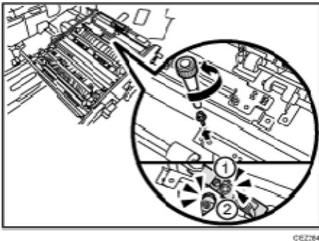
20. Reattach the double-feed sensor with the black screw.
