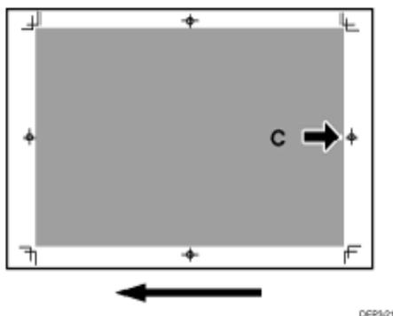
In [Advanced Settings] for the custom paper you are using, adjust the value in 007: [Adj Magnification of Side1 With Feed].
