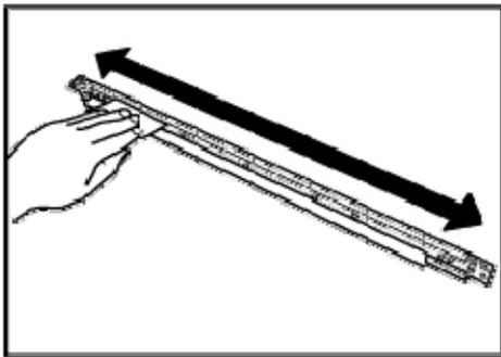
7. Turn the knob while using a dry cloth on the transfer timing idle roller.
