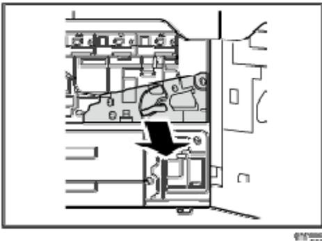
4. Remove the three black screws on the cover plate, and then remove the cover plate.
