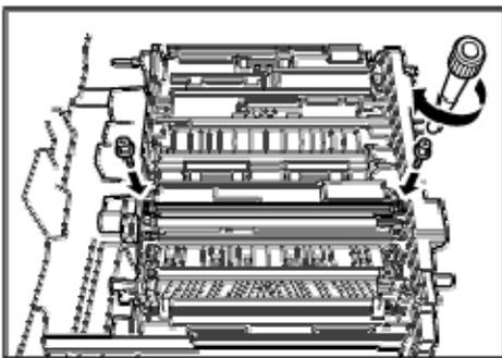
9. Reattach the cover plate with the three black screws.
