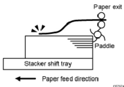
3. The trailing edge of the sheet, while delivered, is left in the paper exit.
