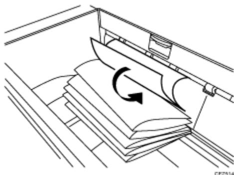
As a bundle is delivered, its folded edge may droop and catch on the stacked bundles, causing the delivered bundle to flip over.
