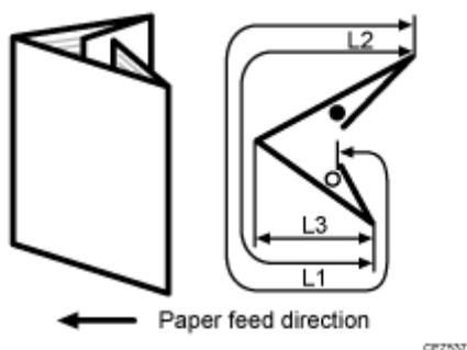
The ○ mark indicates the leading edge (relative to the paper feed direction), and the ● mark indicates the trailing edge.
