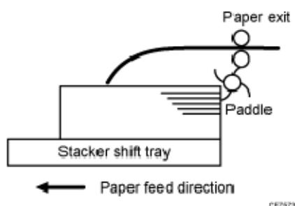
2. The leading edge of the sheet, while delivered, causes strong paper-to-paper friction against the top sheet of the stack. As there is no air gap between the sheets, and the delivered sheet becomes stuck.
