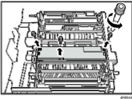
5. Remove the two black screws on the dust catcher, and then remove the dust catcher.
