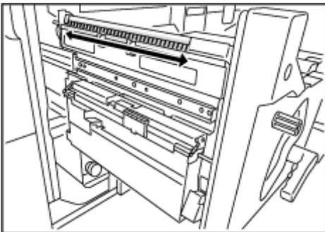
23. Release and pull down duplex transport path plate (Z3).
