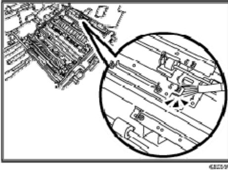
19. Remove the black screw on the double-feed sensor bracket and clean the sensors.
