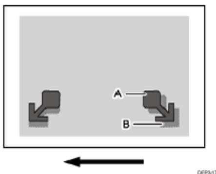
In [Advanced Setting] for the custom paper you are using, select 008: [Adj Magnification of Side2 With Feed].
