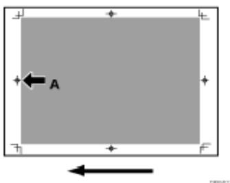
In the [Machine: Image Position] group on the [Adjustment Settings for Skilled Operators] menu, adjust the image position.
