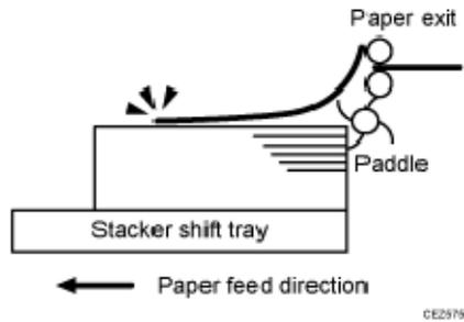
4. The next sheet to be delivered slips under the sheet still in the paper exit and bends back.
