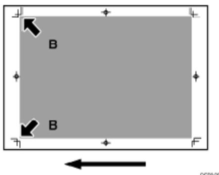
In [Advanced Settings] for the custom paper you are using, adjust the value in 005: [Adj Magnification of Side1 Across Feed].
