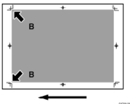
In [Advanced Setting] for the custom paper you are using, select 006: [Adj Magnification of Side2 Across Feed].
