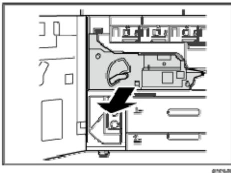
4. **Use a dry cloth to clean the transport belt unit. To clean the sensor, use a blower brush.**
