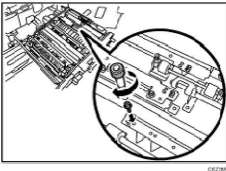
21. Turn the knob B4 on the front while using a dry cloth on the registration timing idle rollers.
