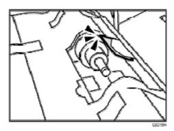
7. Attach the separation roller cover by aligning the tabs.
