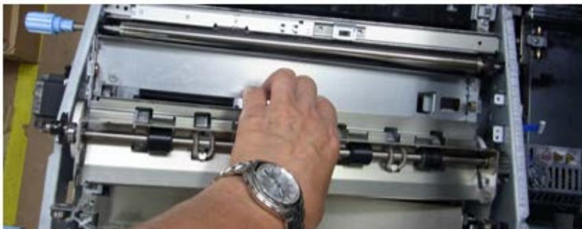
14. Replace the registration gate roller with the modified one in the following procedure.
