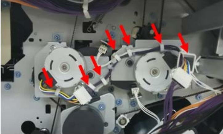
16. Check the connector lift and disconnection of the bifurcated motor
