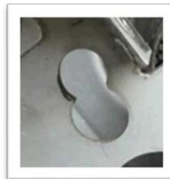
Worn keyhole-shaped slot on the side plate
