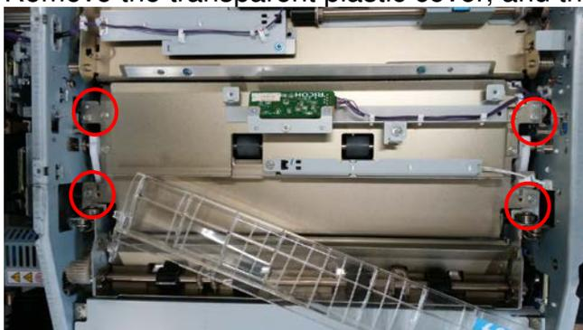
6. Disconnect the sensor connectors and remove the registration timing roller cover.
