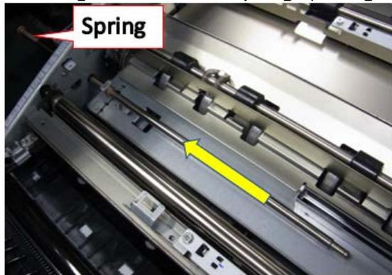
12. Remove the gate home position sensor together with the bracket.
