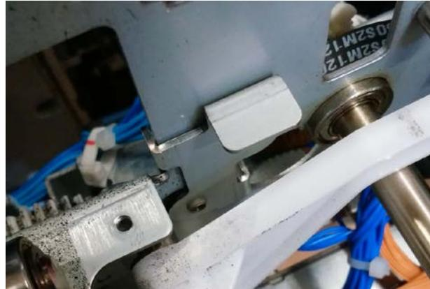
19. Fix the holder and bracket with the screw.
