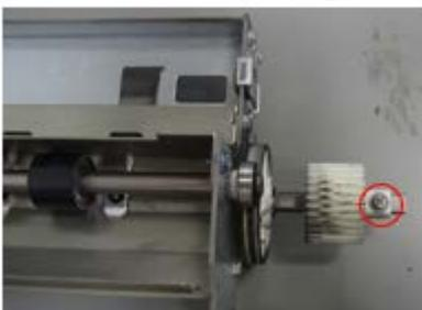
b) Remove the sensor feeler. (M3 screw x 1)
