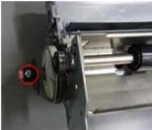
c) Remove the cam. (E-ring x 2)
