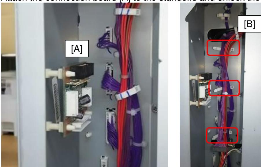
6. Connect the harness to the connection board [A] and the relay connector.
