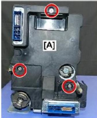
5. At the rear, disconnect the lamp connector bracket at the top [A] and bottom [B] (2screws)
