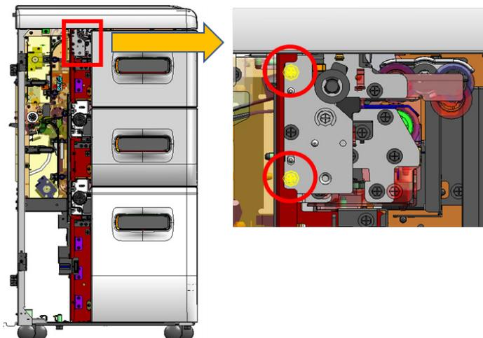
2nd and 3rd paper feed unit: Pull out the PFU along with the brackets (screw x2).
