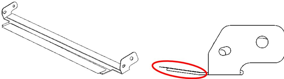
**NOTE: DO NOT** use the new guide plates for thickness 3 or lighter media, to avoid the risk of streaks/bands.
