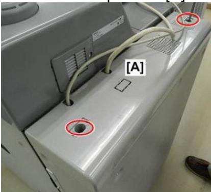
2. Remove the back cover of the controller box. (screw x11)
