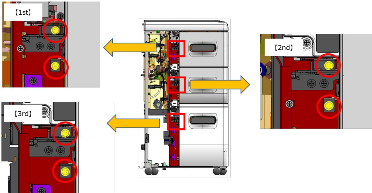
7. 1st Paper Feed Unit: After removing bracket [E], pull out the PFU (screw x2),
