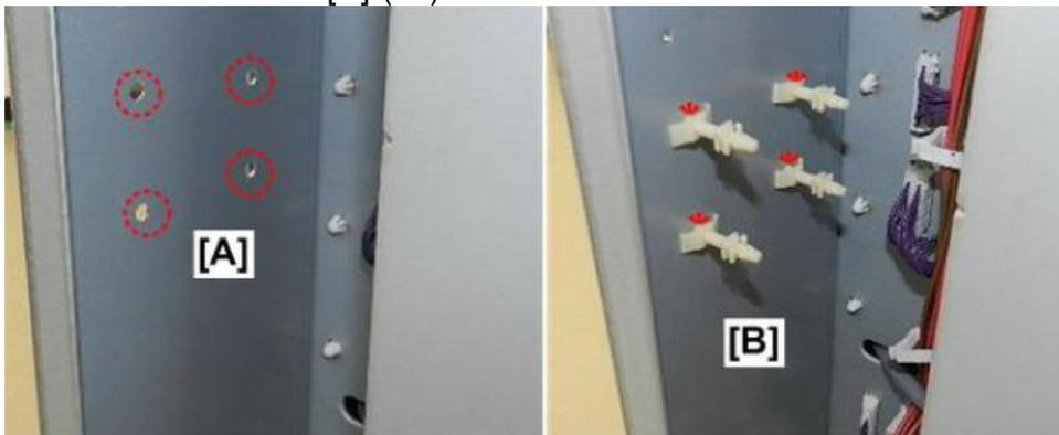
5. Attach the connection board [A] to the standoffs and unlock the harness clamps [B] (x3).
