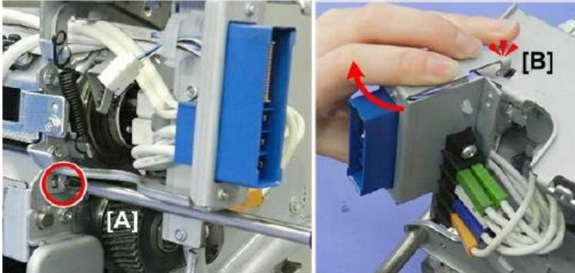
7. At the rear, remove the bracket. (4screws, 1bushing)
