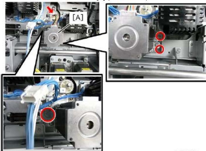
6. Replace Gear [A] (AB014243) and Gear [B] (BB013040) with new ones (E ring x1 screw x1).
