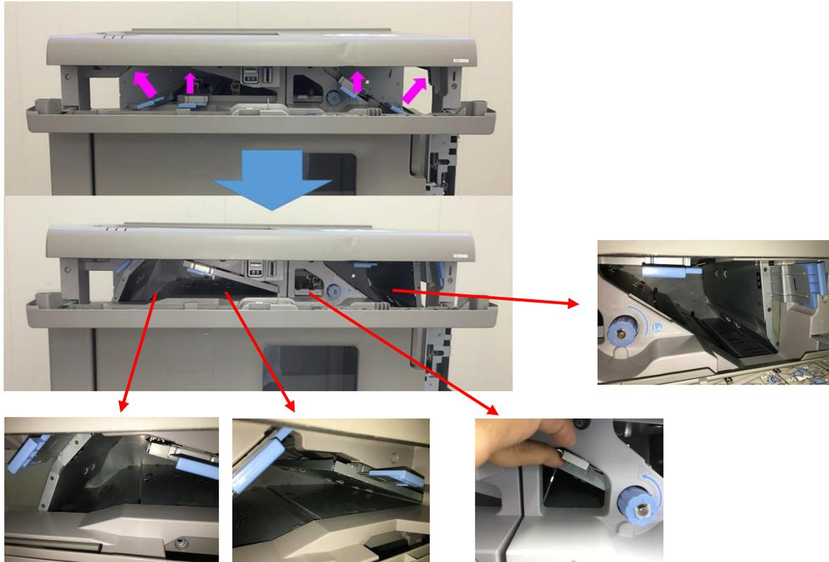
If the stacker can be disconnected, clean the entrance guide plate from the outside (A). However, if the stacker cannot be disconnected, clean the entrance guide plate from the inside (B).
