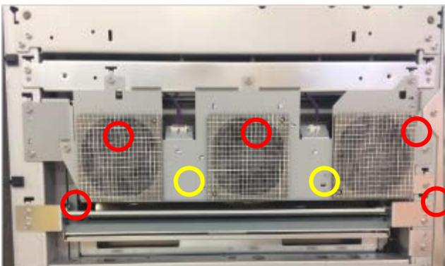
3. Remove the fan cover and fans from the bracket. (Screw x8, Harness clamp x7, Panel mounting adapter x2)
