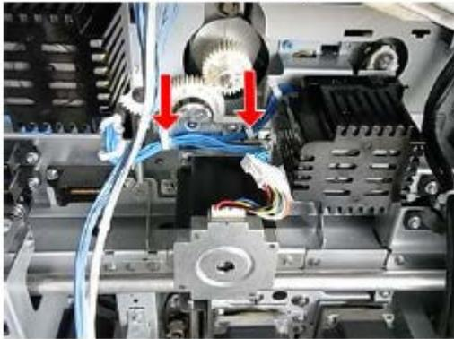
5. Remove the bracket together with the motor (screw x3, connector x1).
