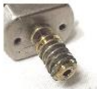
Minimum grease application (0.0161g)
