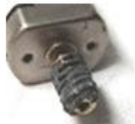
Maximum grease application (0.1287g)
