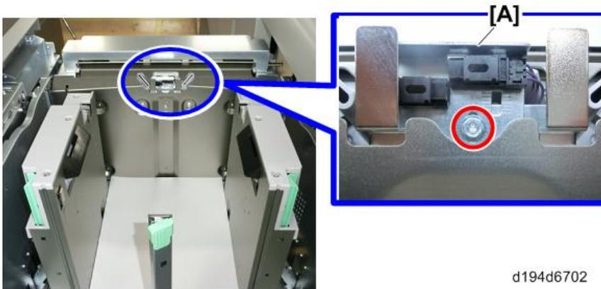
2. Use the scale shown in the diagram below as a guideline to adjust the sensor bracket by sliding up and down.
