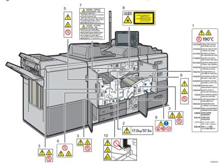
Do not touch the parts a label indicates. The inside and surface of the fusing unit could be very hot. Caution should be taken when removing misfed paper.
