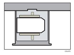
If you are copying or printing onto side-opening envelopes in the  $\Box$  orientation, flaps must be at the right side of the wide LCT or multi bypass tray (Tray 7). If you are copying or printing in the  $\Box$  orientation, flaps must be at the bottom side of the three-tray wide LCT or multi bypass tray (Tray 7). Be sure to load the envelopes with print side face up.
