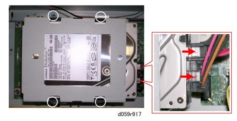
2. Disconnect the HDD bracket (⋛ x4, 록┛ x2).
