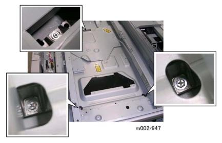
3. Loosen the three screws [B] that hold the laser unit.
