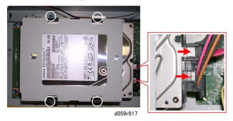
2. Disconnect the HDD bracket (♂ x4, 🗐 x2).
