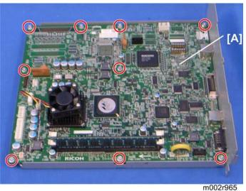
4. Remove the egret controller board [A] from the bracket ( ${\mathscr F}$  x9)
