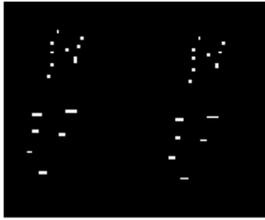
White spots appear as dots or small lines at 314 mm (12 inches) intervals, in the direction of paper feed.
