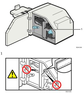
Keep your hands clear of the internal cutting blade when you are removing jammed paper. Not doing so risks injury to your fingers from the cutting blade.
