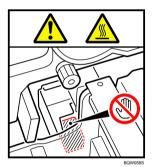
Do not touch the parts a label indicates. The inside of the Multi-Folding unit could be very hot. Caution should be taken when removing misfed paper.
