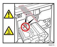
Do not touch the parts a label indicates. The inside of the printer could be very hot. Caution should be taken when removing misfed paper.
