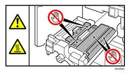
Do not touch the parts a label indicates. The inside of the printer could be very hot. Caution should be taken when removing misfed paper.
