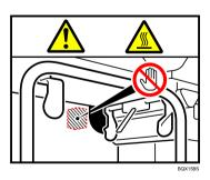
Do not touch the parts a label indicates. The inside of the stacker could be very hot. Caution should be taken when removing misfed paper.
