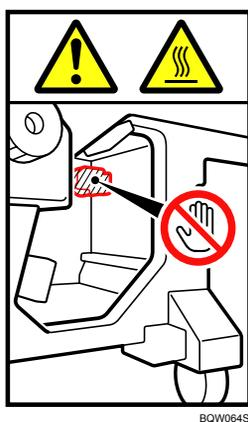
Do not touch the parts a label indicates. The inside of the Multi-Folding unit could be very hot. Caution should be taken when removing misfed paper.
