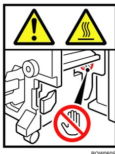
Do not touch the parts a label indicates. The inside of the Multi-Folding unit could be very hot. Caution should be taken when removing misfed paper.
