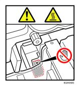
Do not touch the parts a label indicates. The inside of the Multi-Folding Unit could be very hot. Caution should be taken when removing misfed paper.
