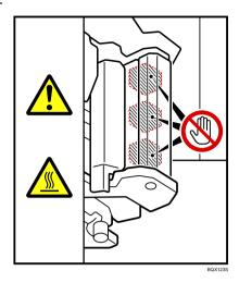
Do not touch the parts a label indicates. The inside of the booklet finisher could be very hot. Caution should be taken when removing misfed paper.
