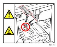
Do not touch the parts a label indicates. The inside of the machine could be very hot. Caution should be taken when removing misfed paper.
