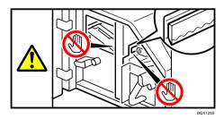
Keep your hands clear of the internal cutting blade when you are removing jammed paper. Not doing so risks injury to your fingers from the cutting blade.
