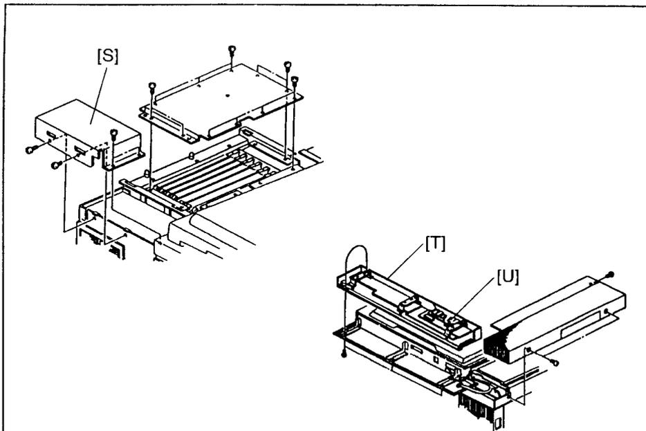
21. Install the interface board cover [S] (4 screws - M4 x 6) and the PCB cover (11 screws).
