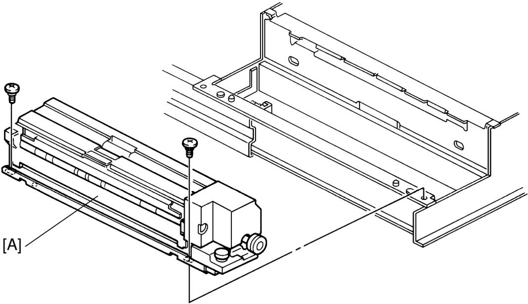
1. Turn the stopper screw counterclockwise, and pull out the transfer belt unit.
