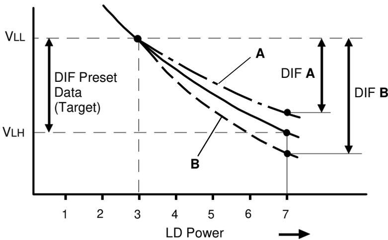
At the factory the targeted DIF data has been preset and is monitored by SPD#120 ~ #123. Before and after each copy job the VLL and VLH patterns are made and are checked by the ID sensor. This difference from VLL to VLH is called the detected DIF data, which is monitored by SPD#125 ~ #128. Then, the detected DIF data is compared with the targeted DIF data:
