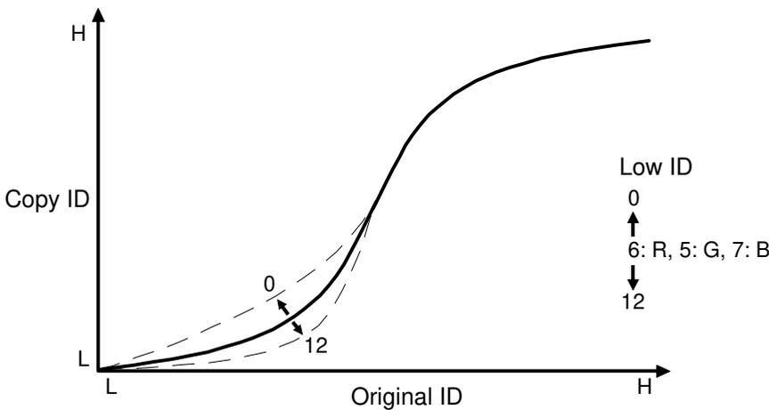
The Low ID mode is used to adjust low image density.
