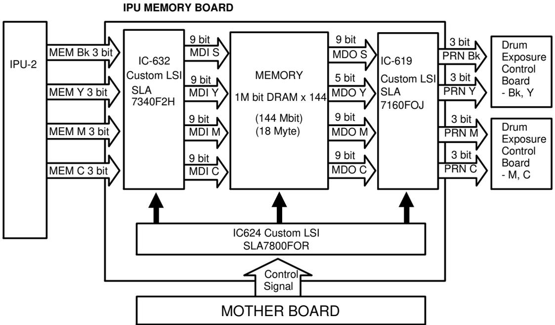
The IPU memory board consists of three custom LSIs and 144 Mbits DRAM (1 Mbit DRAM 144 pcs). This board has the following functions:
