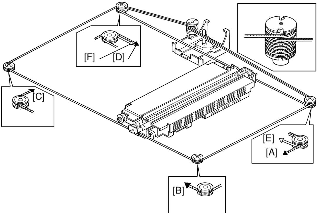
7. Take the dark wire and wind it around the right rear pulley [A], the right front pulley [B], the left front pulley [C], and the left rear pulley [D]. In all cases, make sure the dark wire is in the upper slot of the pulley (see diagram).
