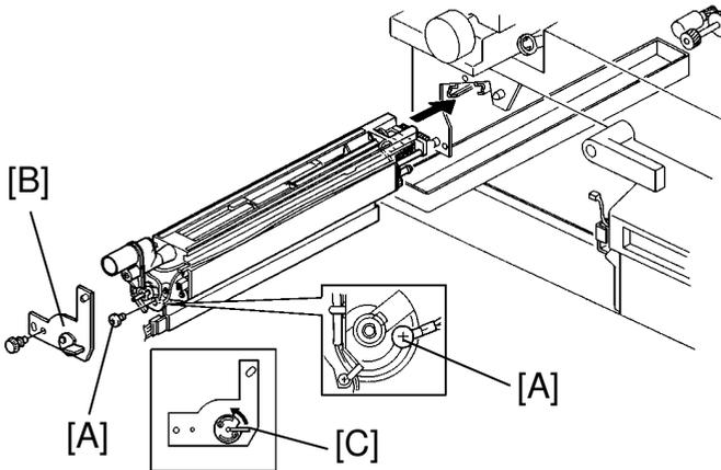
7. Loosen the magnet angle lock screw [A] and set the magnet angle adjuster [B] over the side of the development unit (1 screw).
