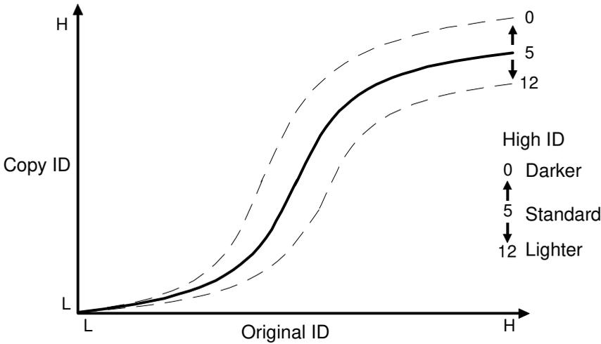
The High ID mode is used to adjust the total image density. The factory setting for each color is 5. In the field, this value should not be changed.
