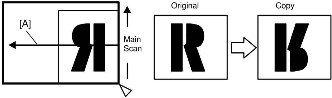
The image is inverted relative to the subscan axis [A].
