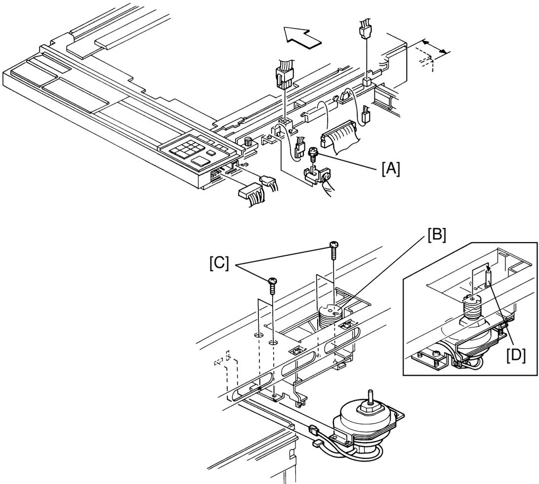
8. Slide the scanner unit 3 centimeters, disconnect all 5 connectors from the scanner unit, and 2 connectors from the operation panel.
