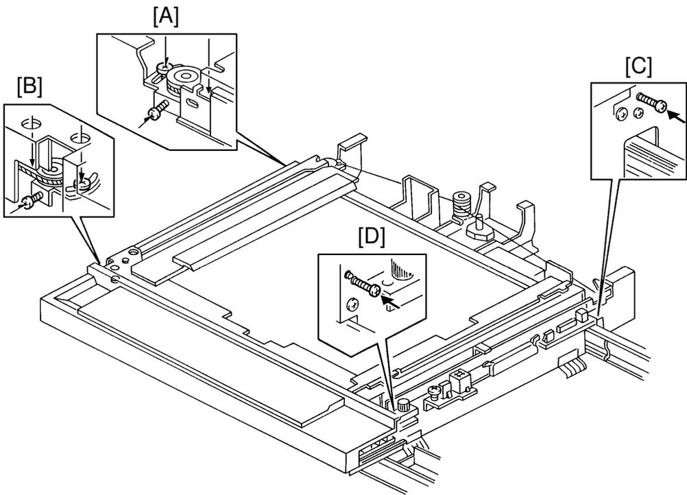
Performing steps 16 to 20 will release the scanner wire tension.
