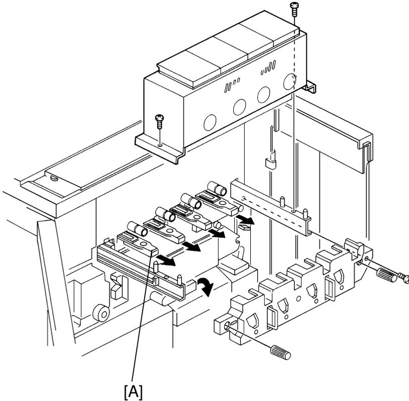
1. Open the front cover and remove the toner tank unit (2 screws).
