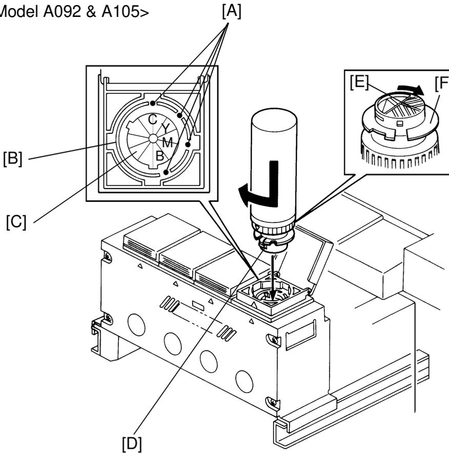
At the top of the toner tank, there is a toner bottle guide which has a positioning pin [A], a notch cut-in [B] and an entrance seal [C].
