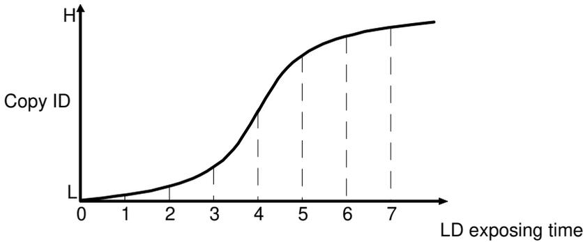
Laser power can be changed over 8 levels by controlling the laser exposure time of each pixel. The relationship between the laser exposure time and the copy ID level is shown in the table. The laser beams for black, magenta, and cyan have 8 levels. However the laser beam for yellow has 4 levels because it is difficult to produce 8 graduations of yellow.
