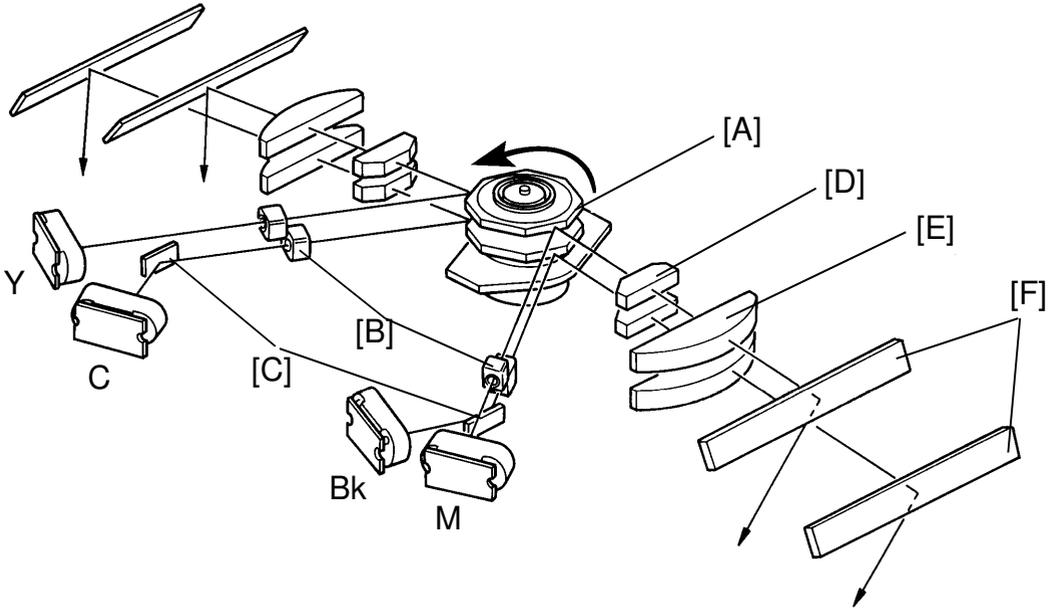
The laser beam path from the laser diode to the OPC drum is shown above.
