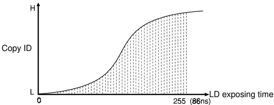
Laser power can be changed over 256 levels by controlling the laser exposure time of each pixel. The exposing time for data 0 is 0s, for data 1 is 2ns, and for data 255 is 86ns. The exposing time between data 1 and 255 is the same interval for each data. The laser beams for all colors have 256 levels.
