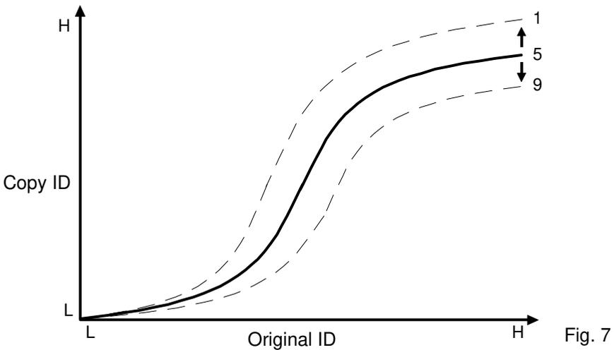
Image density can be adjusted by the Image Density control key on the operation panel. There are 9 density levels (figure 7).
