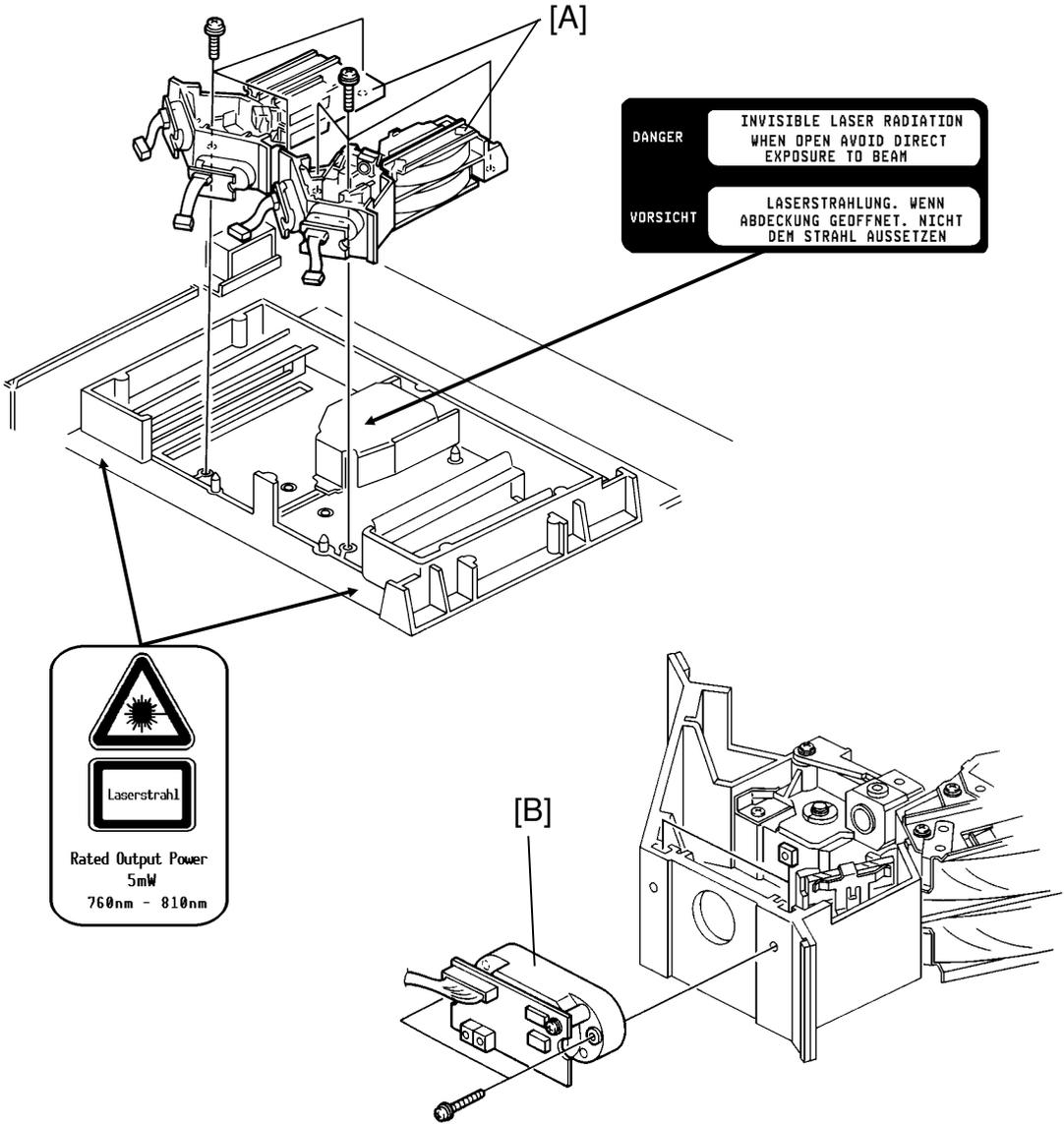
9. Remove the LD control board (6 screws).
