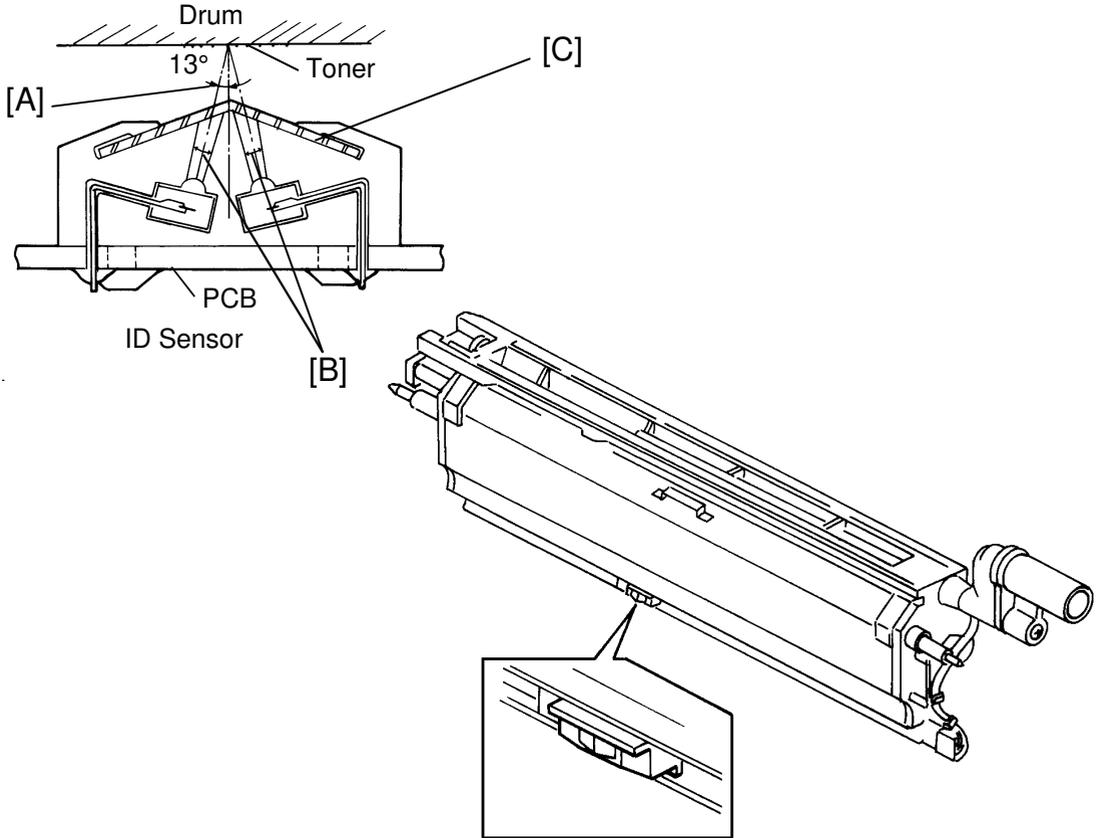
The color toner cannot uniformly reflect the ID sensor light (infrared light), the randomly reflected light from the pattern becomes more as the toner density becomes higher. If the standard type of ID sensor was used in this model, it might mis-detect the image density level on the drum due to the randomly reflected light.
