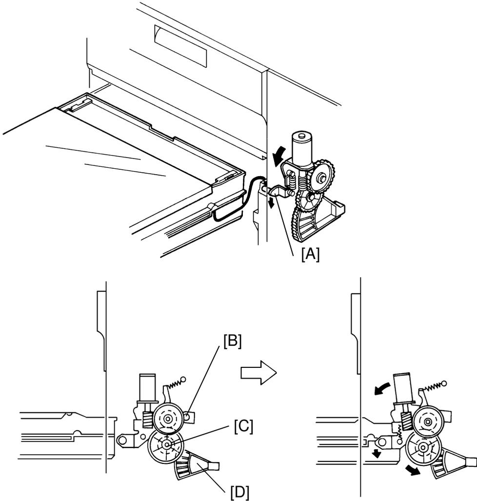
When the cassette is inserted into the copier, the cassette actuator pin [A] is pushed down by the cassette. The lift motor unit then mechanically pivots counterclockwise (looking from the rear of the copier) at point [B] so that the lift gear [C] engages with the sector gear [D].
