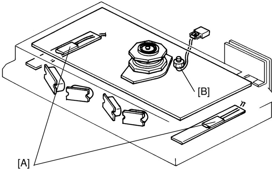
The laser unit has two anti-condensation heaters [A] to prevent condensation from forming on the optical parts (lens and mirrors) and to help prevent any expansion/contraction of the unit due to temperature changes.
