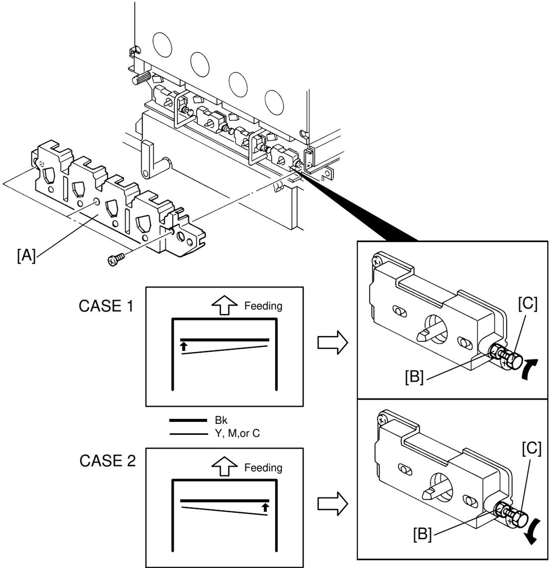
6. Remove the plastic part of the drum unit cover [A].
