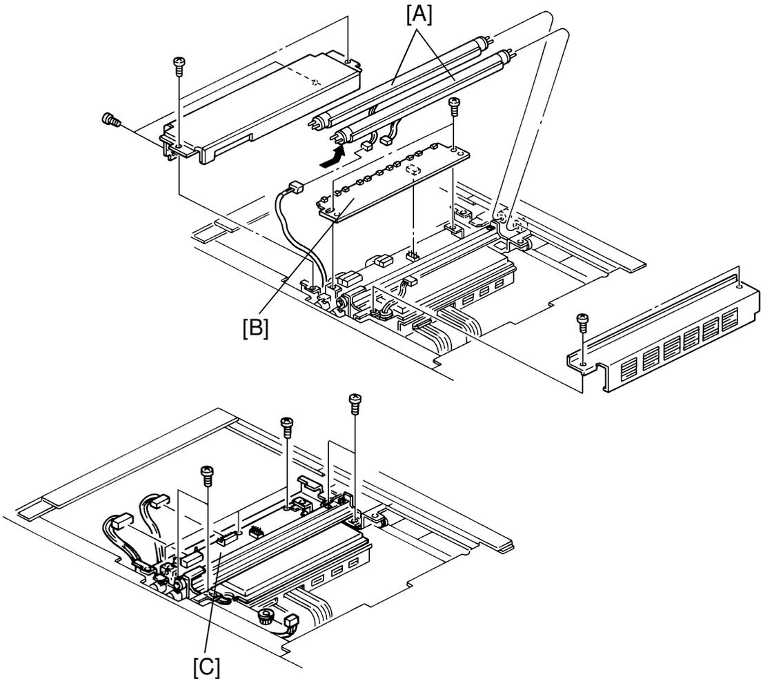
**CAUTION:** For model A092 replace the CCD drive/CCD pre-amp/video processing boards at the same time. These PCBs are a matched set.
