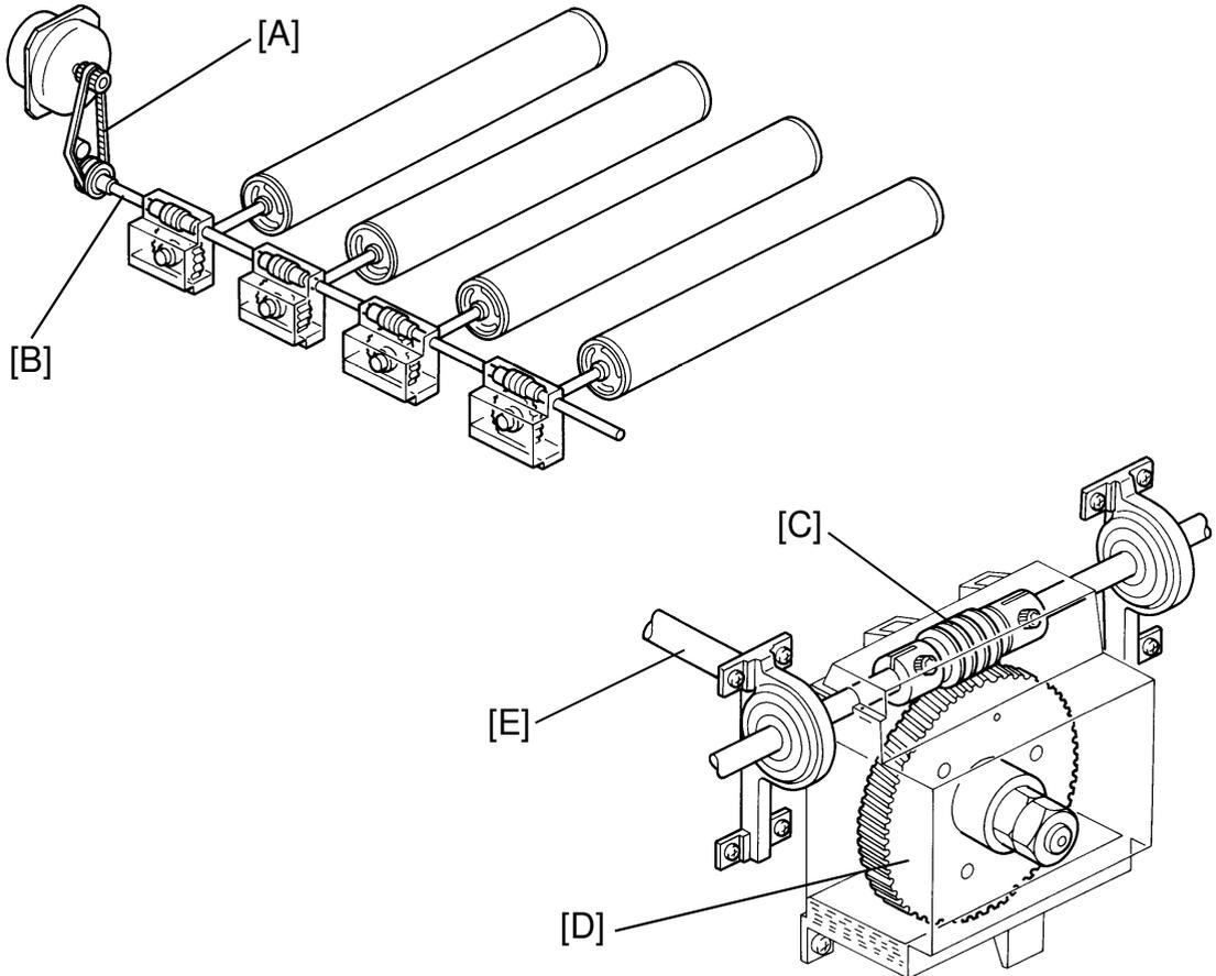
The OPC drum motor drives the 4 OPC drums through the timing belt [A], the worm drive shaft [B], the worm shaft [C], the worm gear [D], and the drum shaft [E]. The OPC drum motor speed is controlled by the motor control board. The speed is 75 mm/sec in standard mode and 37.5 mm/sec in OHP/thick mode.
