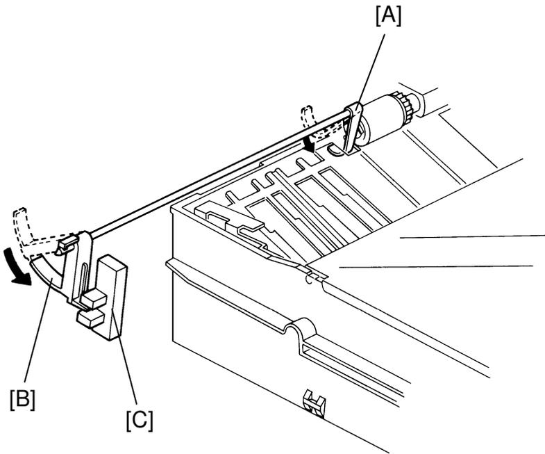
When paper is in the cassette, the paper stack lifts the paper end feeler [A]. When paper runs out, the paper end feeler falls through a groove in the bottom plate and the sensor actuator [B] installed on the end of the actuator shaft blocks the paper end sensor [C]. The paper feed control board detects the paper end condition and lights the "Add Paper" indicator.
