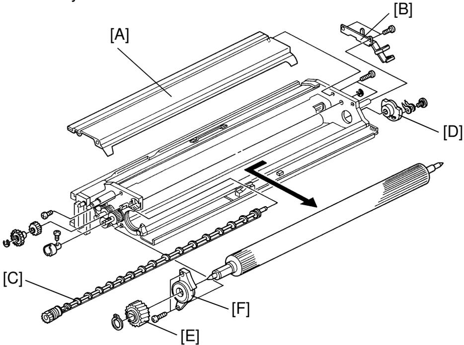
1. Remove the development unit (see Installation Procedure, step 23 to 25).
