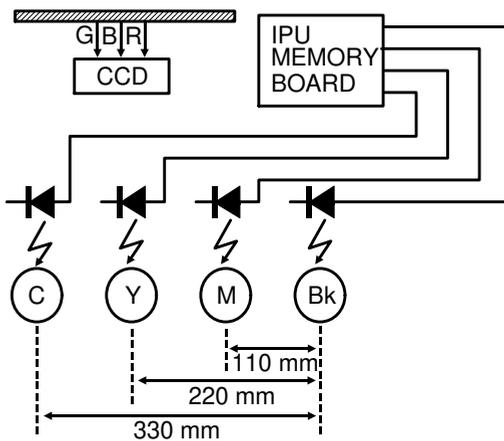
Laser exposure timing for each color is different, because of the tetradrive layout. Laser exposure for each color is done at intervals (see figure). Black is exposed immediately but the video data for magenta, yellow and cyan must be stored in memory.
