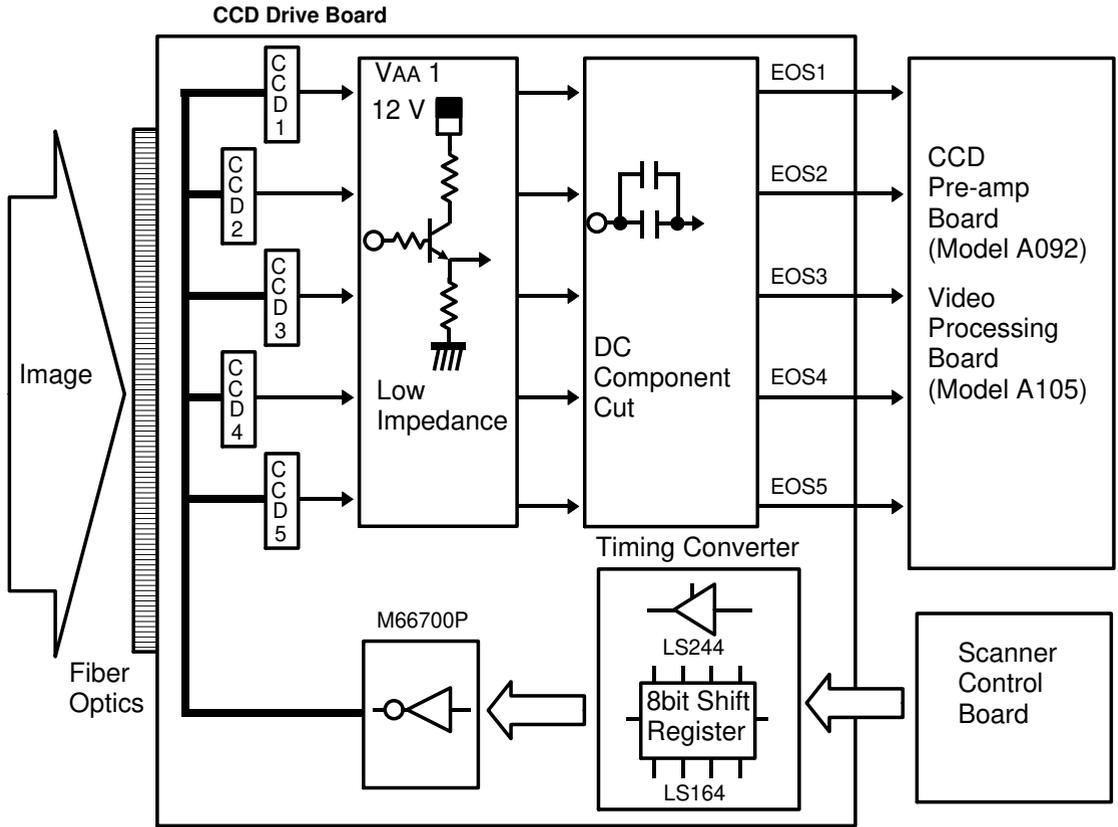
The timing signals for the CCDs come from the scanner control board. The timing converter transfers them to the 5 CCDs.
