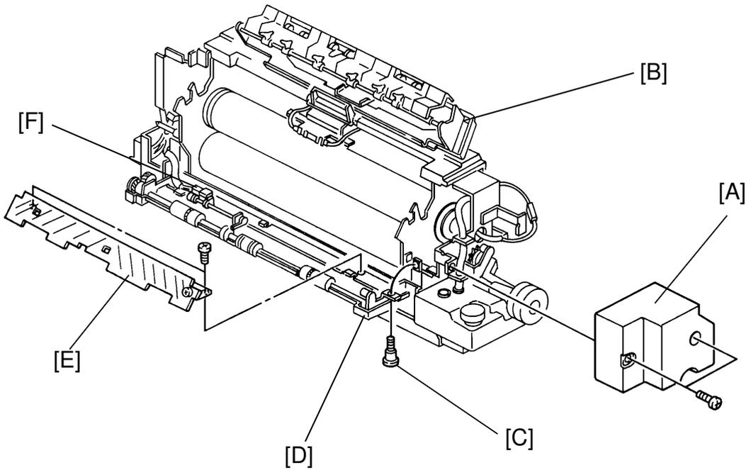
1. Remove the cover [A] (two M4 x 8 screws).
