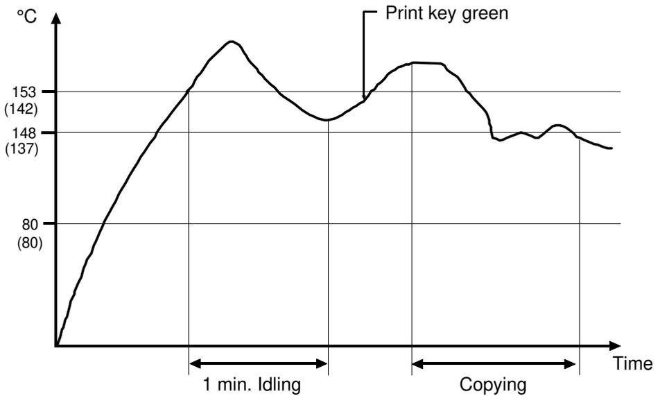
To control the temperature of the hot roller, the fusing lamp is turned off and on by the SSR (Solid State Relay).
