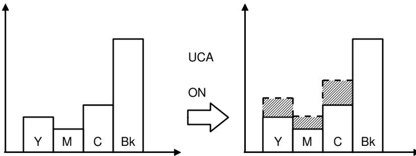
Using only UCR processing, the copy image lacks depth. So, a specified ratio of toner is added for each color (yellow, magenta, cyan). The amount of additional toner added for each color is in proportion to the overall color's density.
