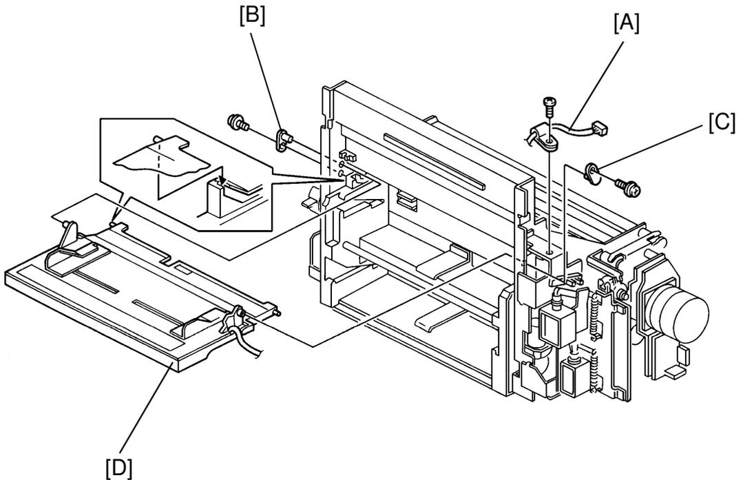
1. Pull the paper feed unit out and remove the lower side cover (5 screws).
