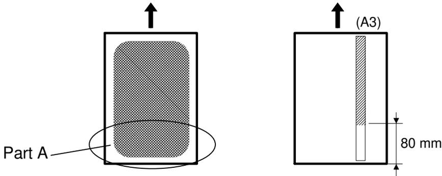
Perform "PAPER FEED UNIT POSITIONING ADJUSTMENT" when the following phenomenon occurs on the copy image.
