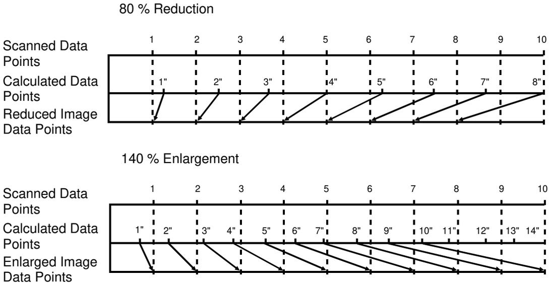
Reduction and enlargement in the sub scan direction is done by changing the scanner speed. However, reduction and enlargement in the main scan direction is handled by IPU board 1.
