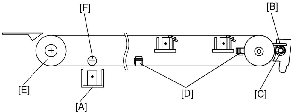
After cyan toner is transferred to the paper, the transfer belt must be cleaned both electrically and physically.
