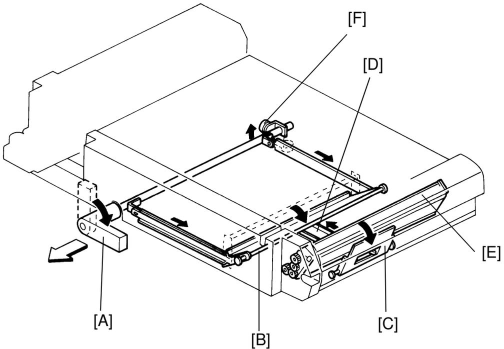
When the transfer unit handle [A] is turned clockwise, the transfer belt arm [B] is pulled down via the unit's linkage. The transfer belt is then released from the drums. Since the belt cleaning unit arm [C] is connected with the belt arm another linkage [D], the belt cleaning unit [E] is also released from the transfer belt.
