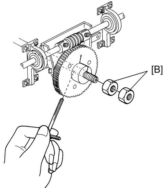
**CAUTION: When turning the worm gears, turn them counterclockwise only. Turning them clockwise will damage the cleaning blades.**
