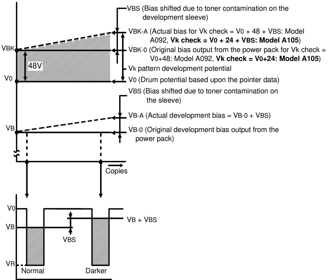
The development roller sleeve is subjected to toner contamination (or residual toner remaining on the development sleeve) which will gradually increase as the number of copies made is increases. Corresponding to this increase of toner contamination, actual development bias [VB-A] is increased, and is higher than the bias output from the power pack [VB-0]. This shifted voltage from VB-0 to VB-A is named VBS.
