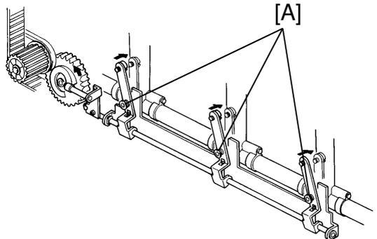
**Drum Drive Gears and Transfer Belt Drive Gears**
