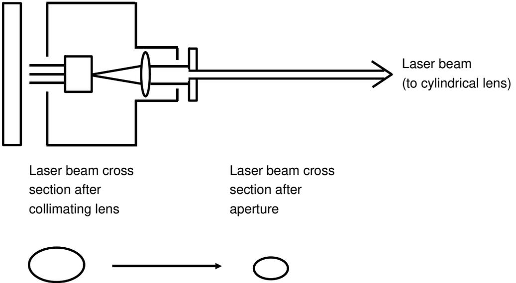
Each LD unit (Bk, M, Y, and C) consists of the LD (laser diode), aperture, collimating lens, and LD driver board.
