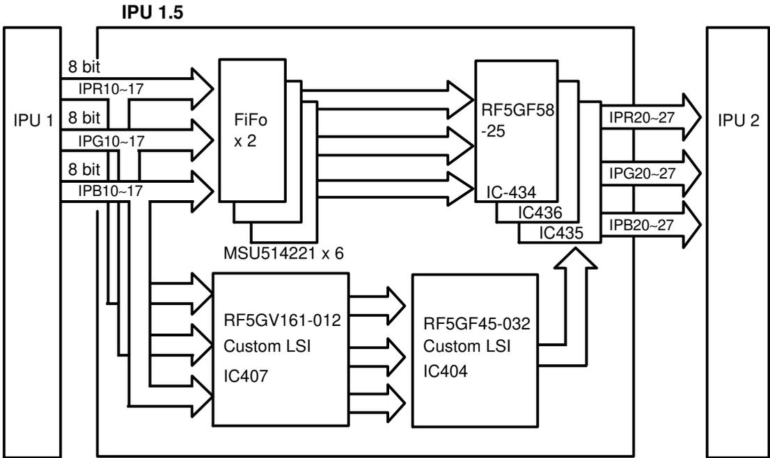
The IPU board 1.5 uses 5 custom LSIs to process the video data. These LSIs perform the following functions:
