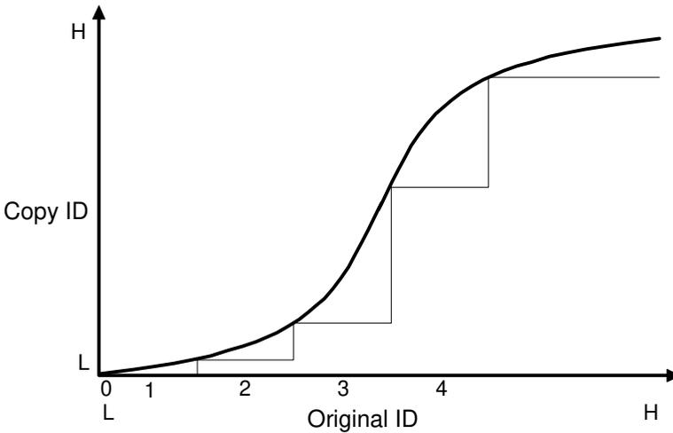
Instead of being distributed over a 64-level range (256 level range for model A105), image density is distributed over a 4-level range. This gives the copy image a poster effect.
