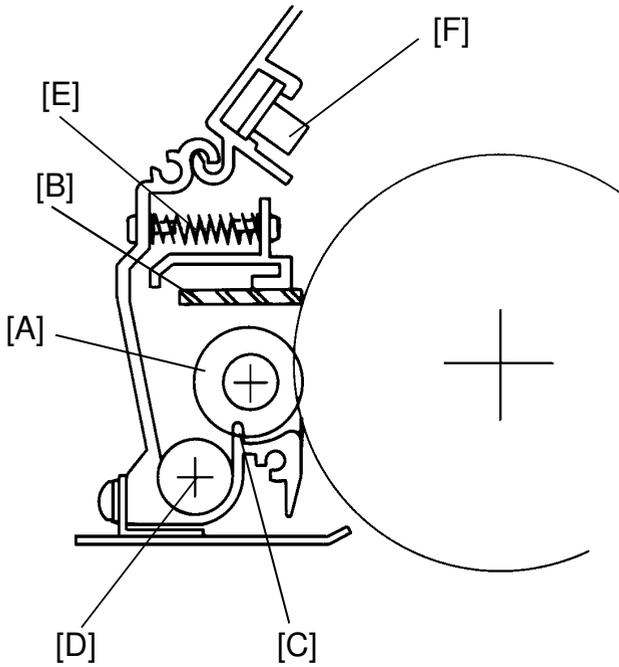
Drum cleaning is accomplished by the cleaning brush [A] and the cleaning blade [B]. This mechanism is very much like other PPCs.
