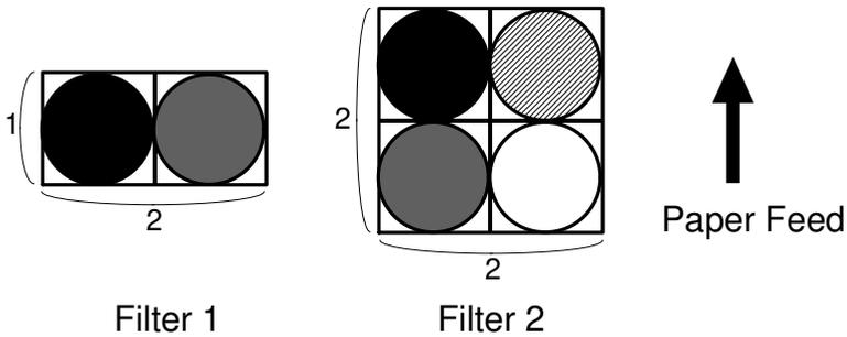
Dither processing is not adopted on this model. This is because one pixel can range over 256 gradations (or shades) for black, magenta, yellow, and cyan. This means that a 256 gradation full color image can be out put without dither processing. However, to make a smoother looking image 2 digital filters are adopted on this model.
