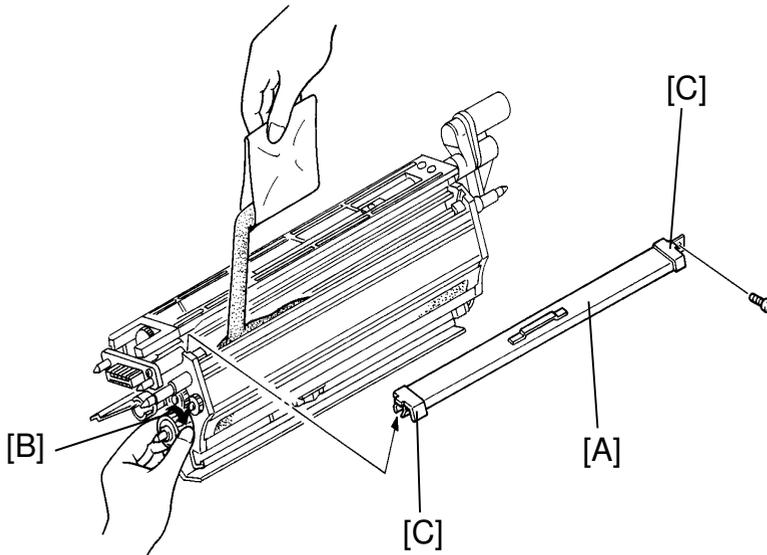
29. Remove the development unit upper cover [A]. (1 screw: for model A105 only)
