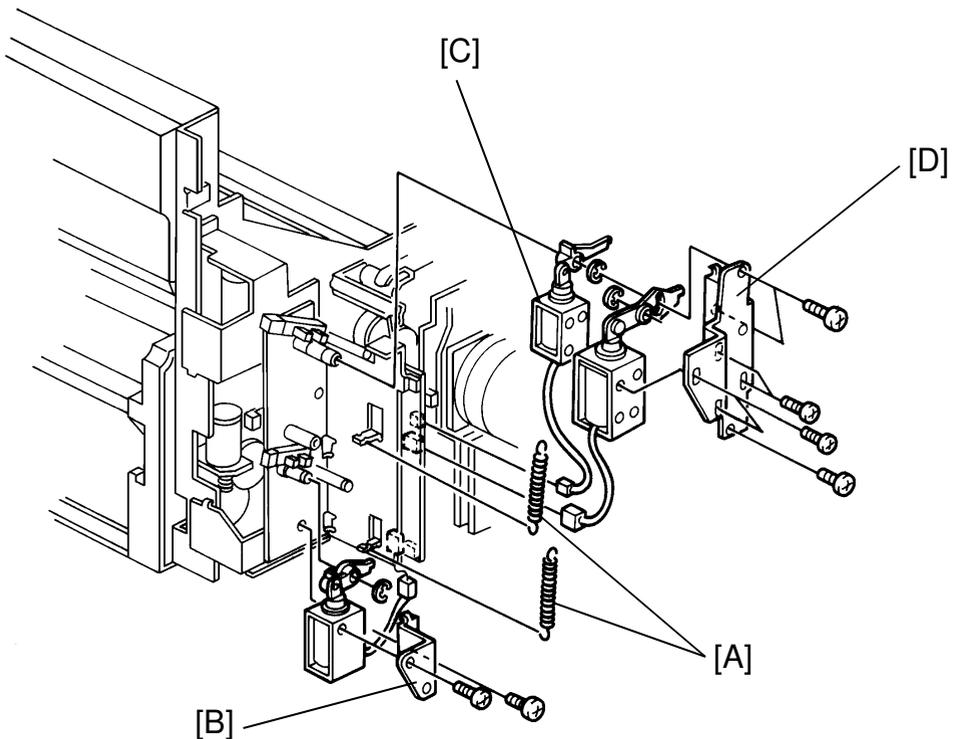
There are two pick-up solenoids and one by-pass solenoid.
