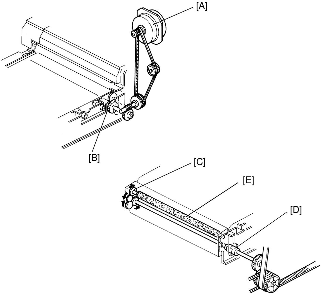
This model uses an independent dc servo motor for transfer belt drive. This is necessary because precise speed control of the transfer belt is required. The rotation of the transfer belt drive motor [A] is transmitted to the transfer drive roller [B] through a timing belt and gears.
