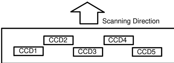
CCD2 and CCD4 scan the image earlier than CCD1, CCD3, and CCD5, because of the CCD layout. The data transfer timing of CCD2 and CCD4 is delayed by buffers (LS244) to match them with the timing of CCD1, CCD3, and CCD5.
