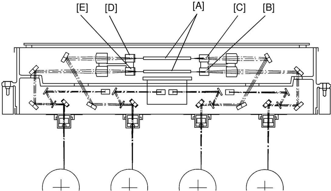
This model uses four laser diodes to produce an electrostatic image on four OPC (organic photoconductor) drums. The LD control board converts image data from the drum exposure control board into laser pulses and the optical components direct these pulses to the OPC drum.
