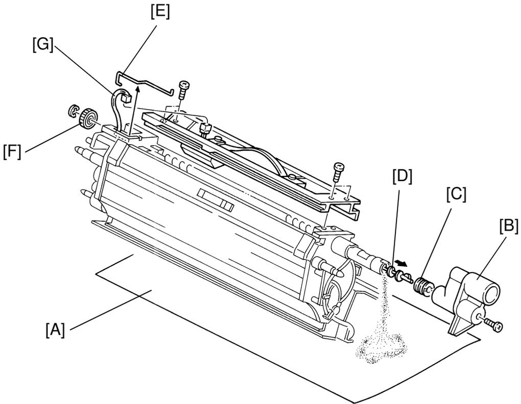
1. Remove the ID sensor before removing the development unit from the machine and put it on the development unit stand.
