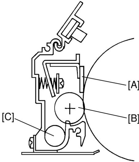
Cleaning mechanism has been changed from that of model A092. For model A092, the trailing blade cleaning mechanism is used. For model A105, the counter blade cleaning mechanism is adopted to remove the new type toner (6.4 $\mu$ m diameter). The only difference is in the way the cleaning blade [A] contacts the drum. The counter-blade mechanism achieves a high reliability (20K PM).
