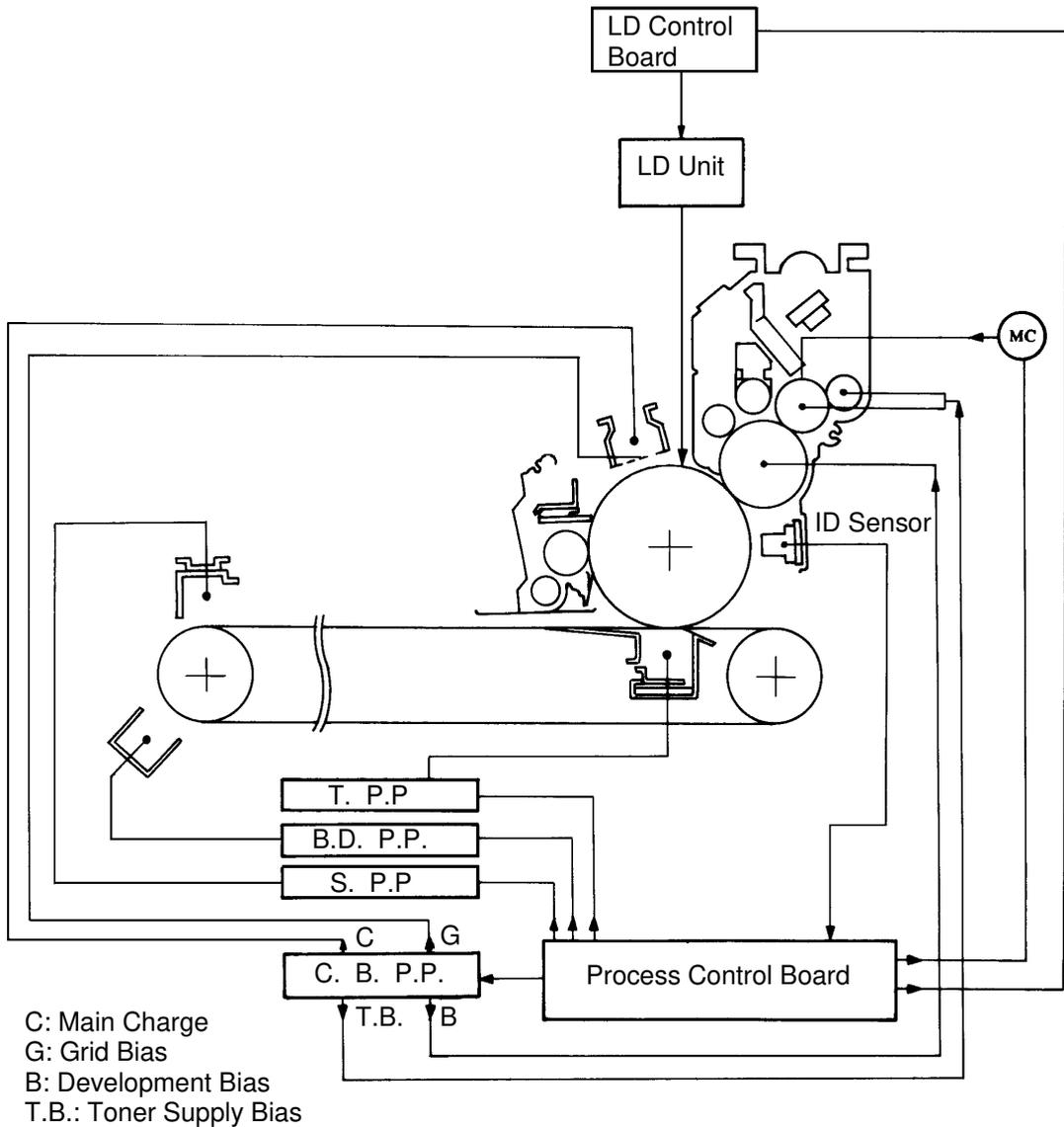
The process control board serves the following two functions to maintain proper copy quality:
