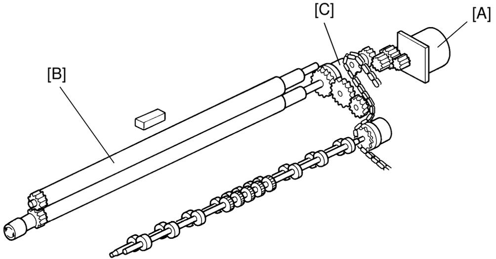
The paper feed motor [A] drives the registration rollers via the drive chain, gears, and the registration clutch.
