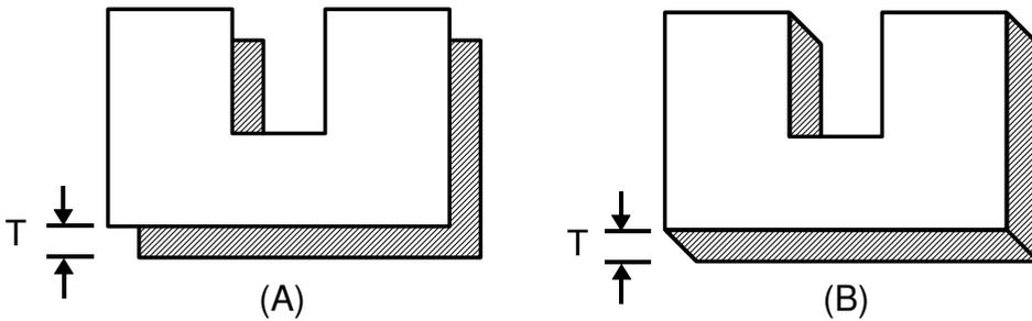
There are two shadowing functions: off-set shadowing (A) and block shadowing (B).
