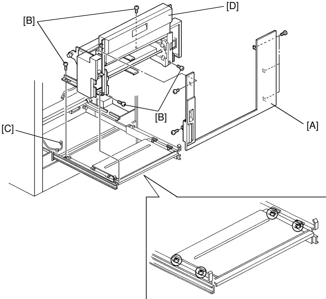
1. Pull the paper feed unit out and remove the lower side cover [A] (5 screws).
