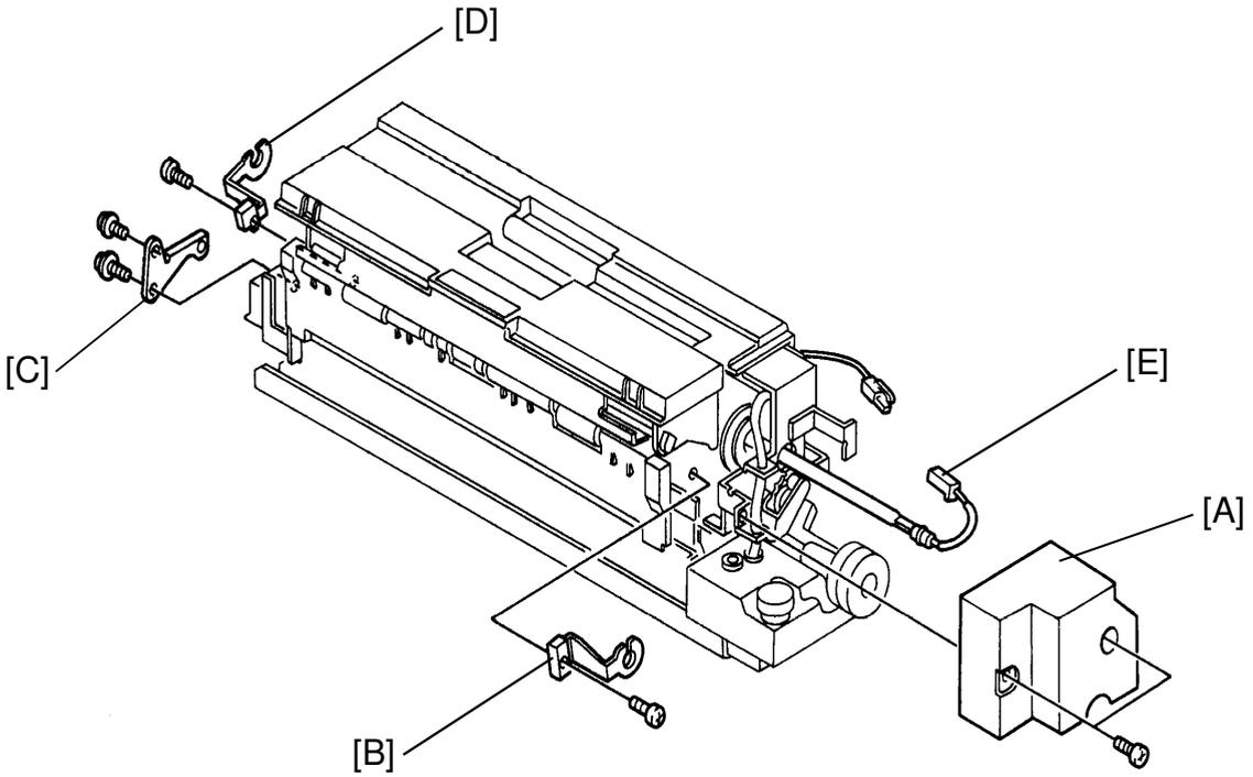
1. Remove the cover [A] (two M4 x 8 screws).
