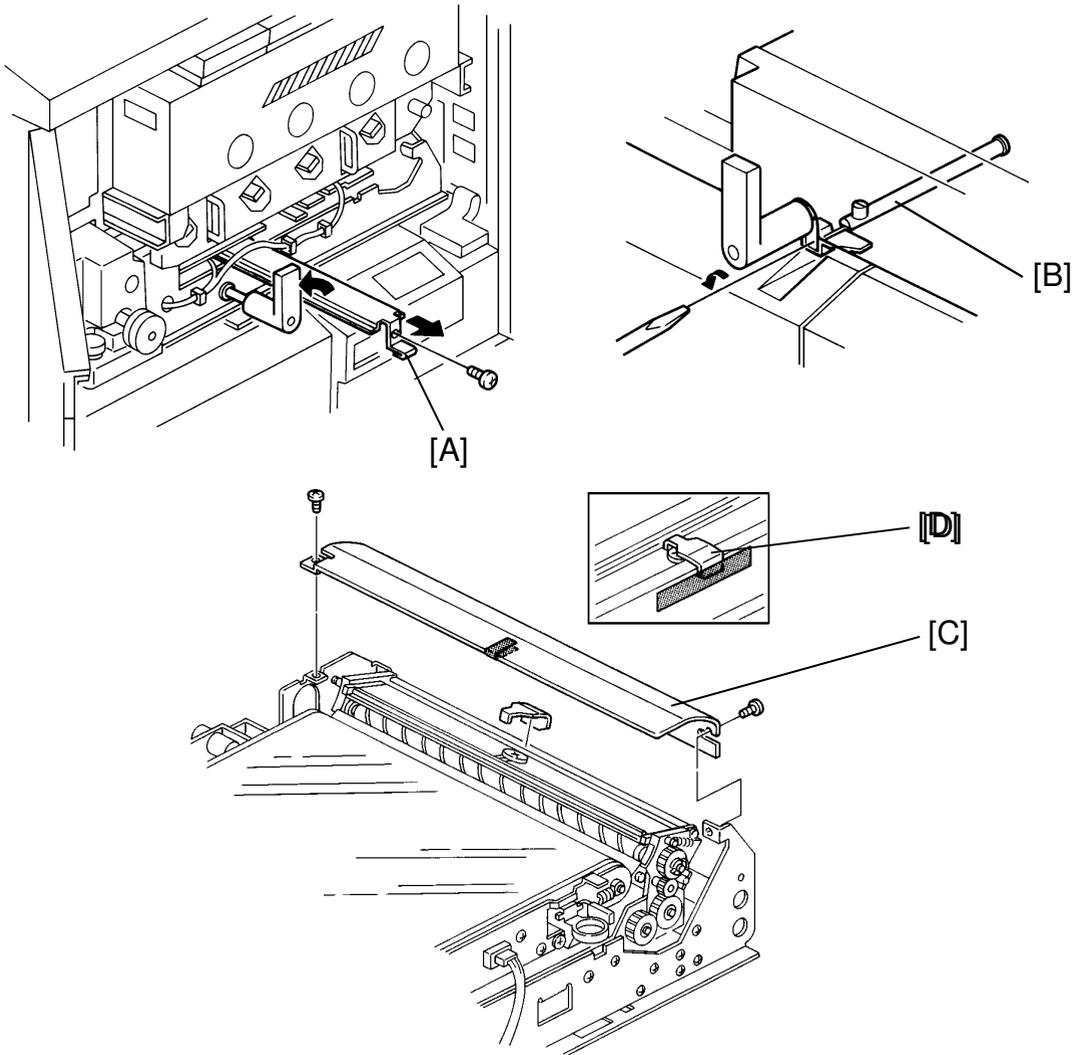
10. Turn handle B1 back to its original position and remove the shipping stay [A] (1 screw).
