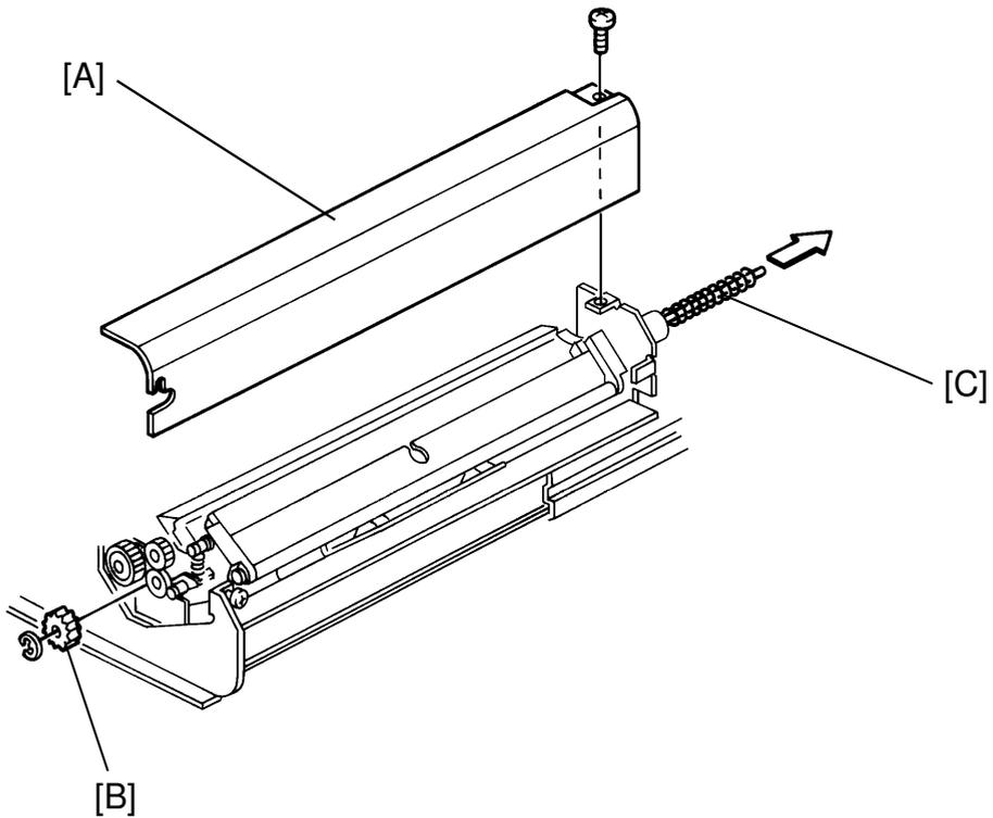
1. Remove the transfer unit (see Transfer Unit Removal).
