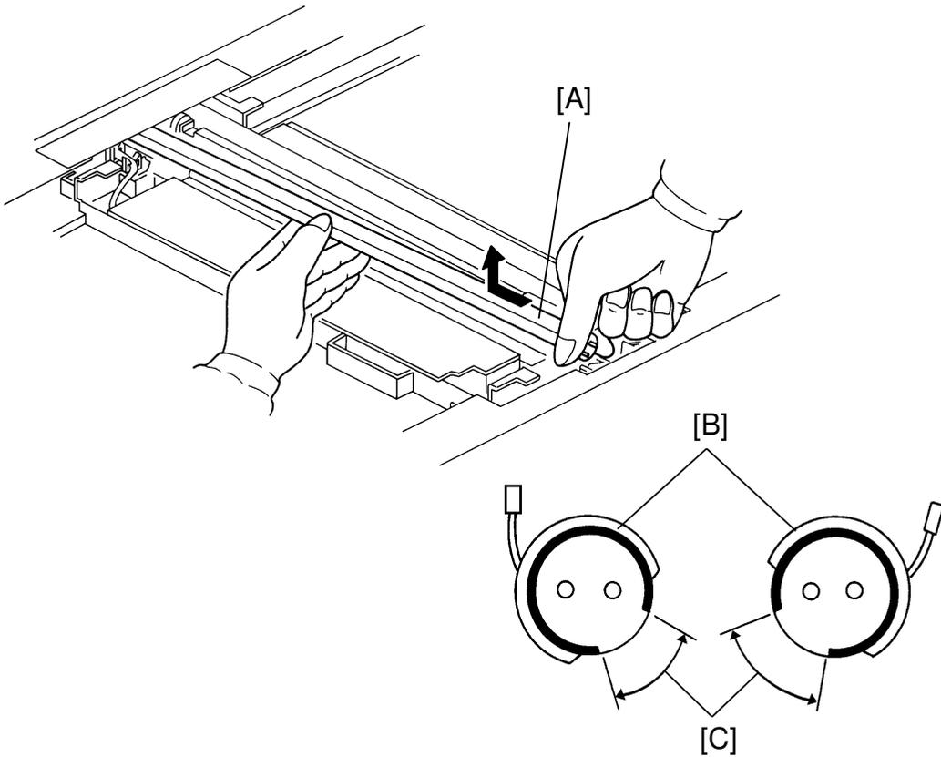
4. Remove the 2 exposure lamp and heater assemblies [A] (1 connector each).
