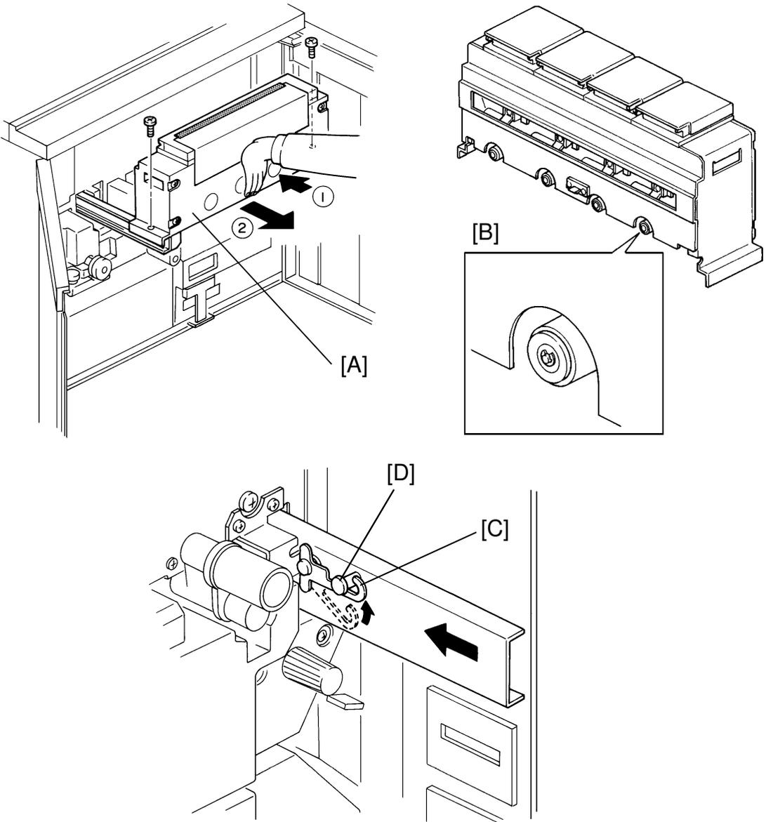
17. Push the center of the toner tank unit [A] to slide the unit out and remove the unit (2 screws and padding).
