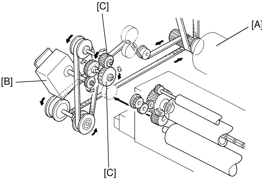
In copying, the rollers in the fusing unit are driven by the main motor [A]. The power of the main motor is transferred to the fusing unit as shown in the illustration by the black (↑) arrows. As the gears [C] have one way clutch mechanism, the main motor power does not transfer to the fusing idling motor [B].
