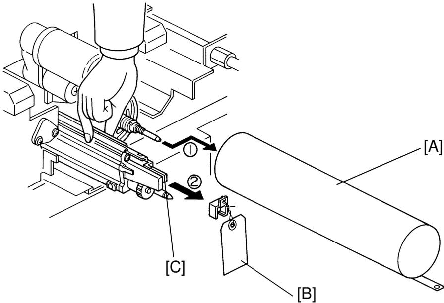
27. Pull the drum protective sheet [A] off the drum.
