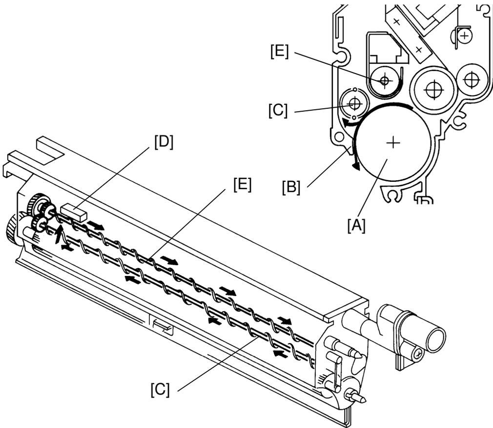
In model A092, only two augers and one permanent magnet serve for both cross-mixing and for agitating the developer.
