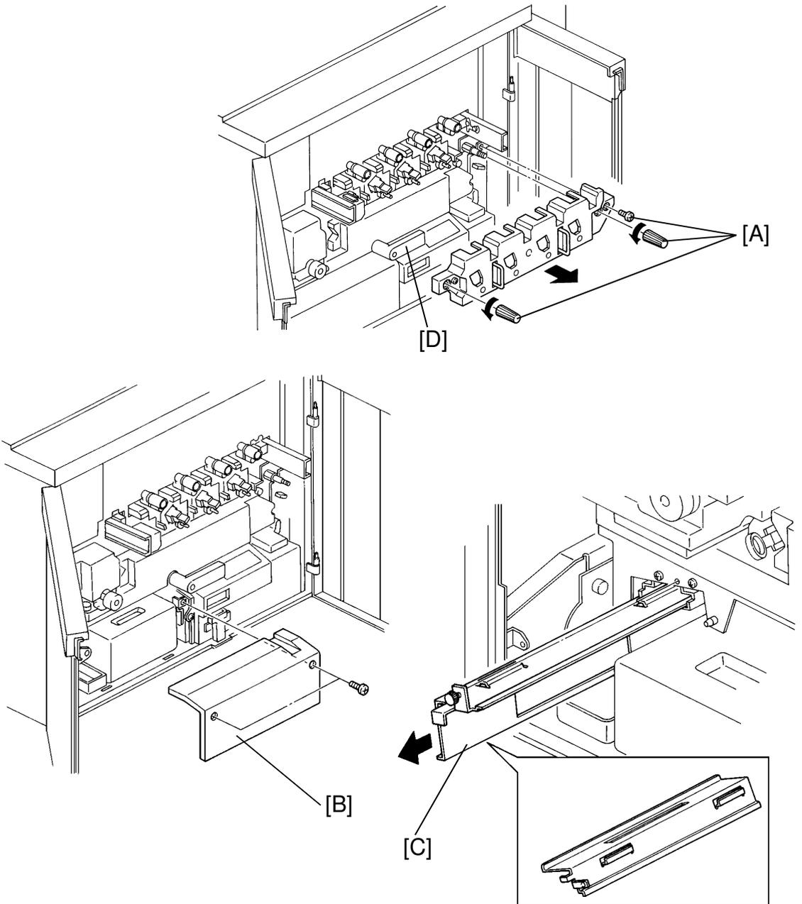
20. Turn the B1 lever [D] clockwise and remove the screws [A] (2 knob screws, one ordinary screw) and slowly pull the drum unit cover.
