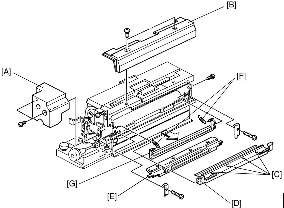
1. Remove the cover [A] (two M4 x 8 screws).
