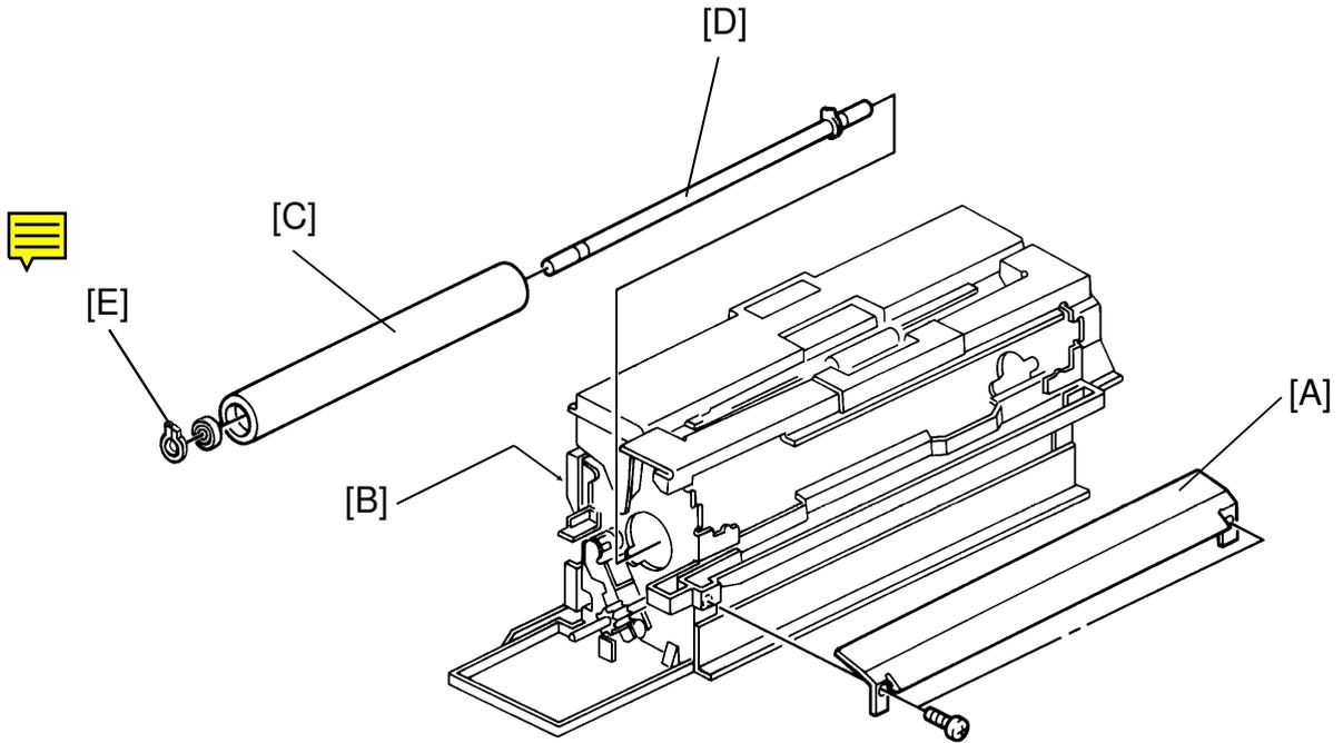
1. Remove the hot roller (see hot roller replacement).
