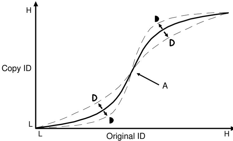
Contrast can be adjusted by the contrast keys on the left side of the operation panel. The contrast of each color (Y, M, C, Bk) can be adjusted independently over 9 levels. The slope of the line in the graph changes, but stays centered around point A. (A: 32 of 64 graduation steps)
