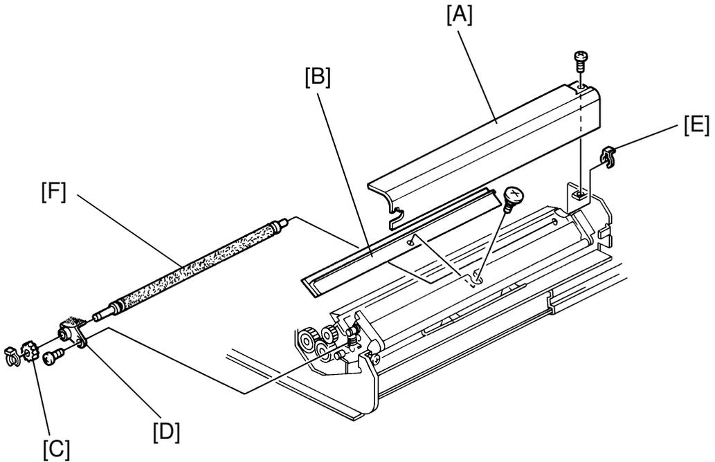
1. Turn the transfer unit stopper lever counter-clockwise using a minus screwdriver pull the unit all the way out.
