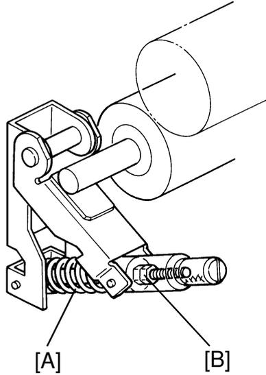
The pressure roller is pressed upwards by the pressure spring [A]. The pressure is adjusted by the position of the nuts [B]. If the nuts are lowered, the pressure is decreased; on the other hand, if the nuts are raised, the pressure is increased. The pressure is checked by measuring the nip band on an OHP sheet (Folex 100).
