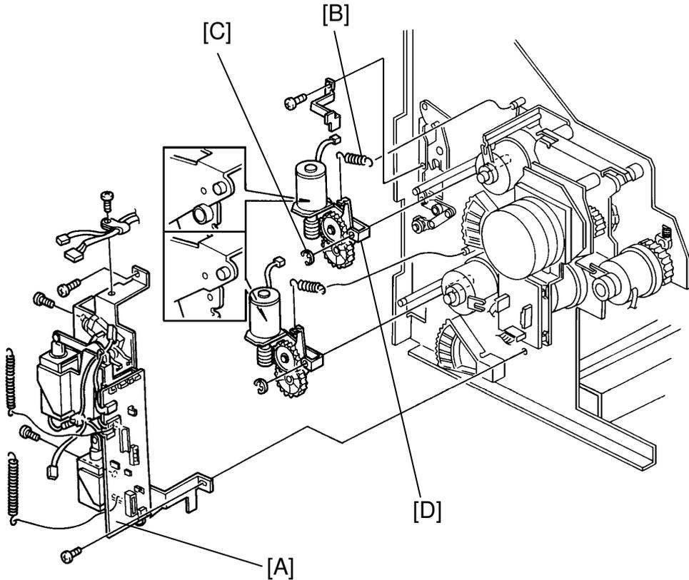
Be careful to distinguish the upper paper lift motor and gear assembly from the lower one. The assembly brackets do not match and are not interchangeable.
