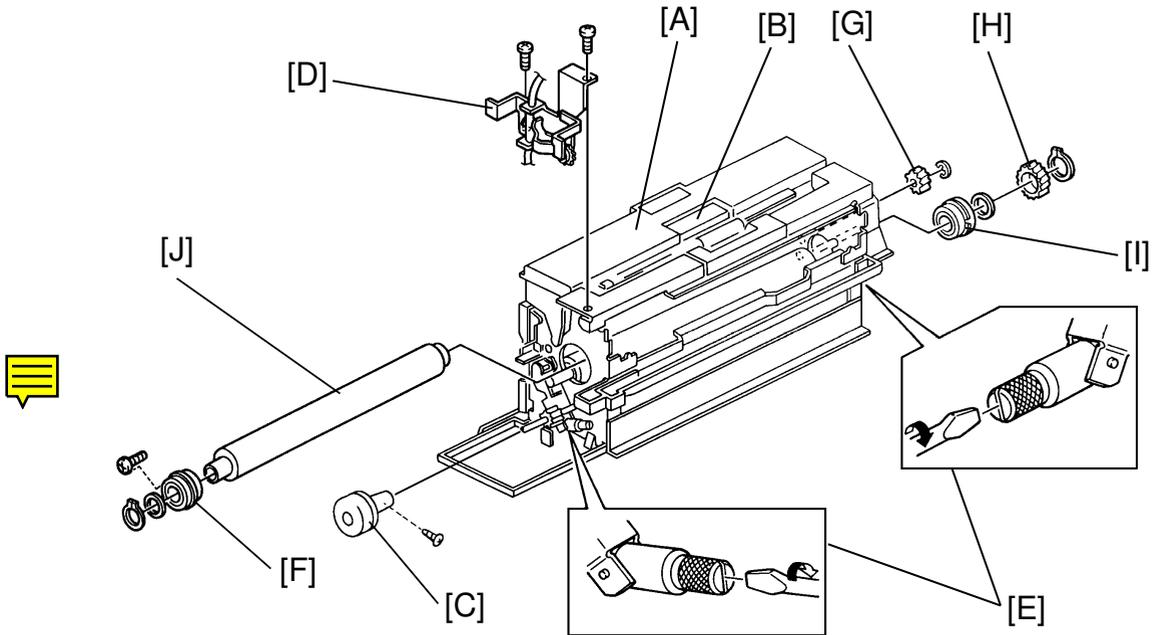
1. Remove the fusing heater (see fusing heater replacement).
