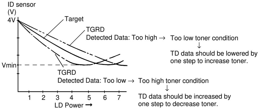
TD check is necessary after new developer installation. After the reset of the process data such as the pointer, ND, CD, and other data, a free run and a self check is performed at least four times.
