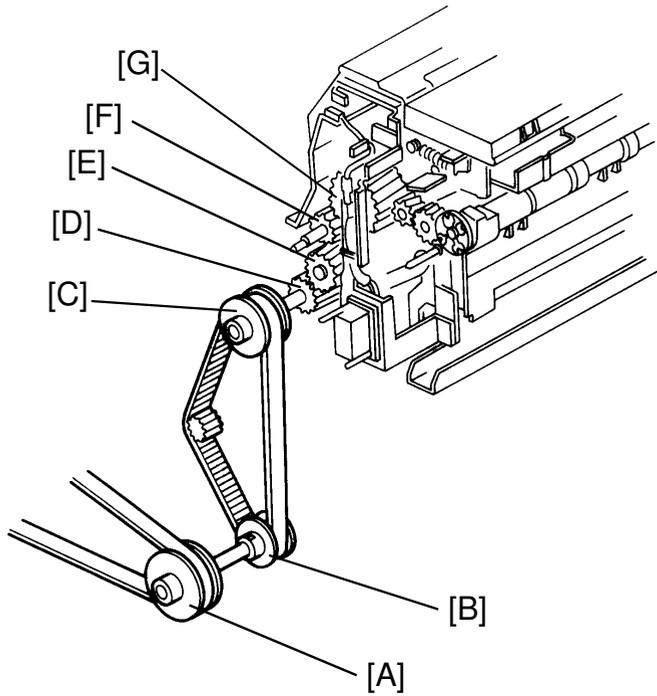
The rollers in the fusing unit are driven by the main motor. The torque of the main motor is transferred to the fusing unit through the following gears and belts: timing belt, pulley 47T [A], pulley 25T [B], timing belt, pulley 35T [C], 1st drive gear 21Z [D], 2nd drive gear 27Z [E], idle gear 20Z [F], fusing roller 45Z gear [G].
