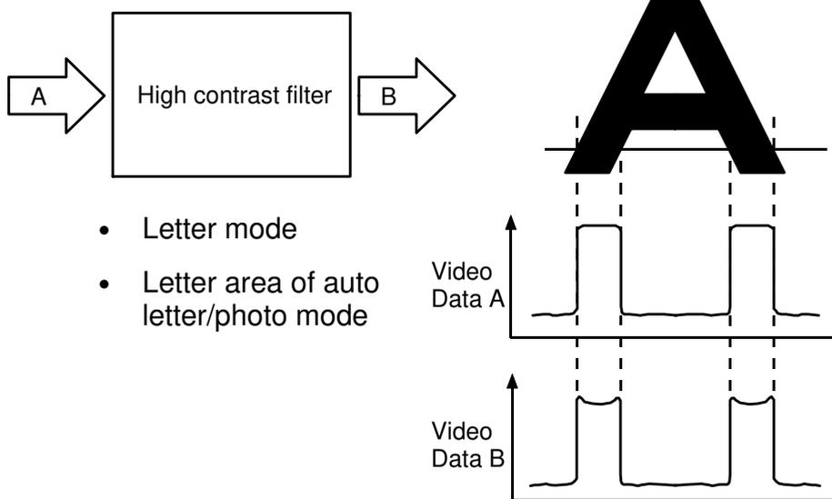
There are two MTF correction functions. One function is a smoothing filter used in photo and the letter/photo modes. The smoothing filter is also used on the photo area when in the auto letter/photo mode. The other function is a high contrast filter used in letter mode and used on the letter area when in auto letter/photo mode.
