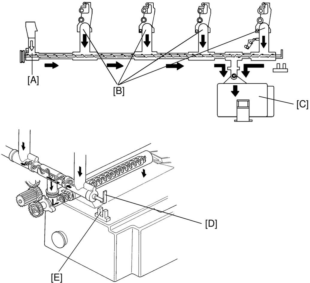
The toner collected during transfer belt cleaning [A] and the toner collected during drum cleaning for each color [B] is transported to the toner collection bottle [C].
