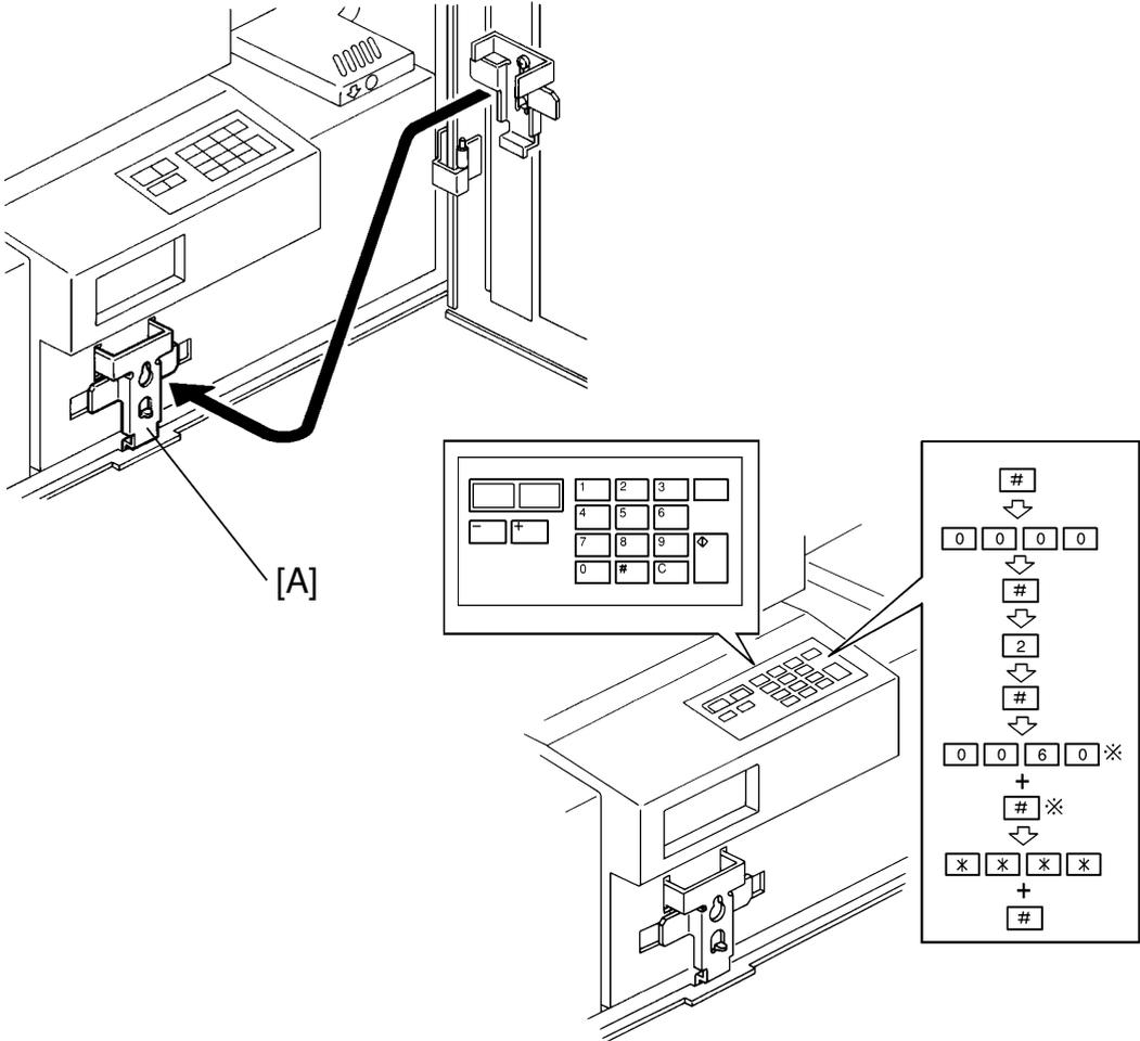
**NOTE:** For a new machine, the access code to SP TEST/DATA Modes is set to "0000" at the factory. At the machine installation, enter your own number using SP Data Mode No. 60. The number set must be recorded for the next access. It is impossible to monitor the access code set once it has been set. It is recommended that the service center use a single standard code.
