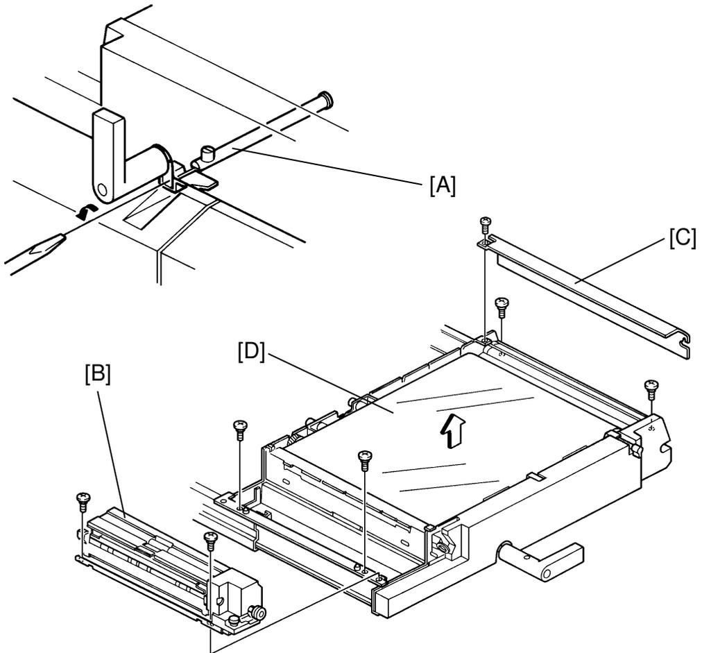
1. Turn the transfer unit stopper lever [A] counter-clockwise using a minus screwdriver and pull the unit all the way out.
