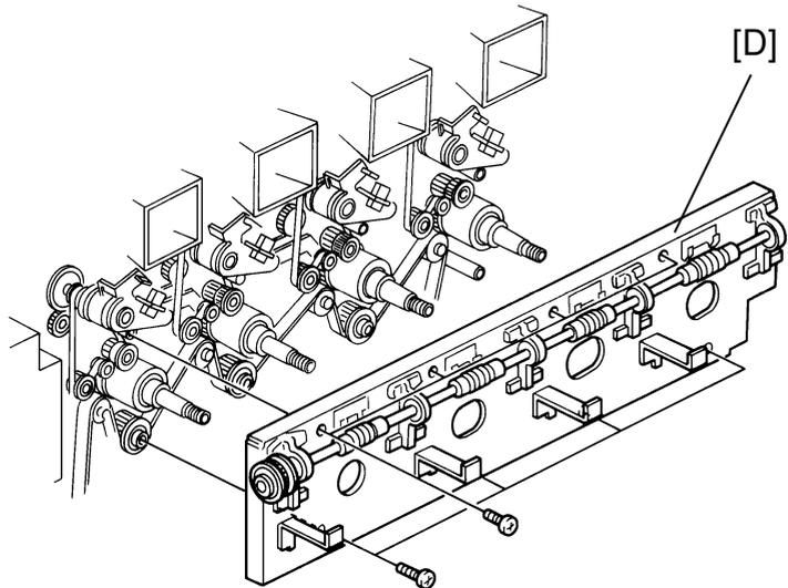
**CAUTION:** Put the worm gears removed in step 8 on a sheet of clean paper or a cloth to prevent them from getting dust or scratches.
