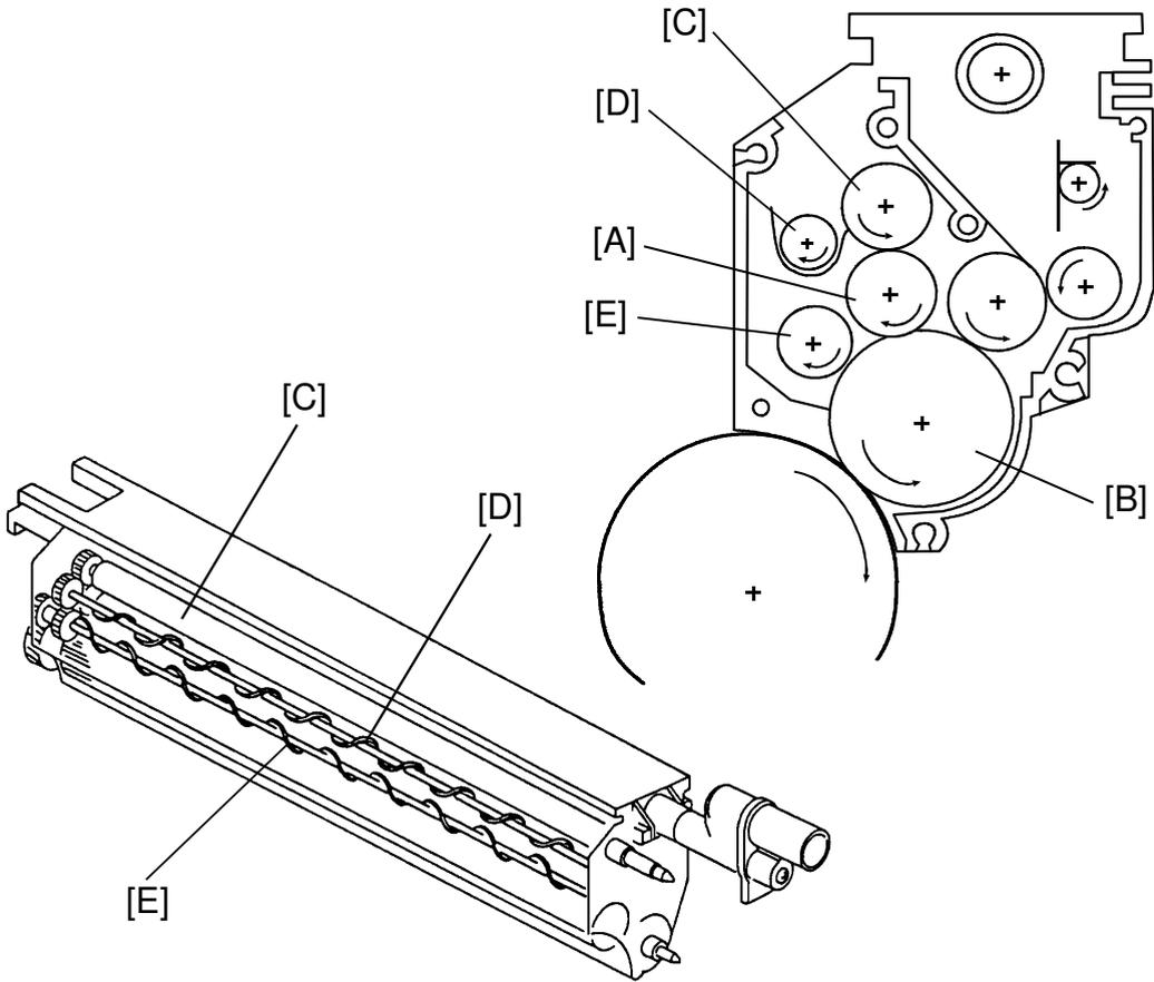
To achieve good copy quality, the development sleeve speed is reduced to half, as explained in the previous section. The rotation speeds of the other rollers in the development unit are also reduced, and this causes insufficient developer mixing. To power up the mixing function, two additional rollers (the upper and lower transfer roller) are adopted.
