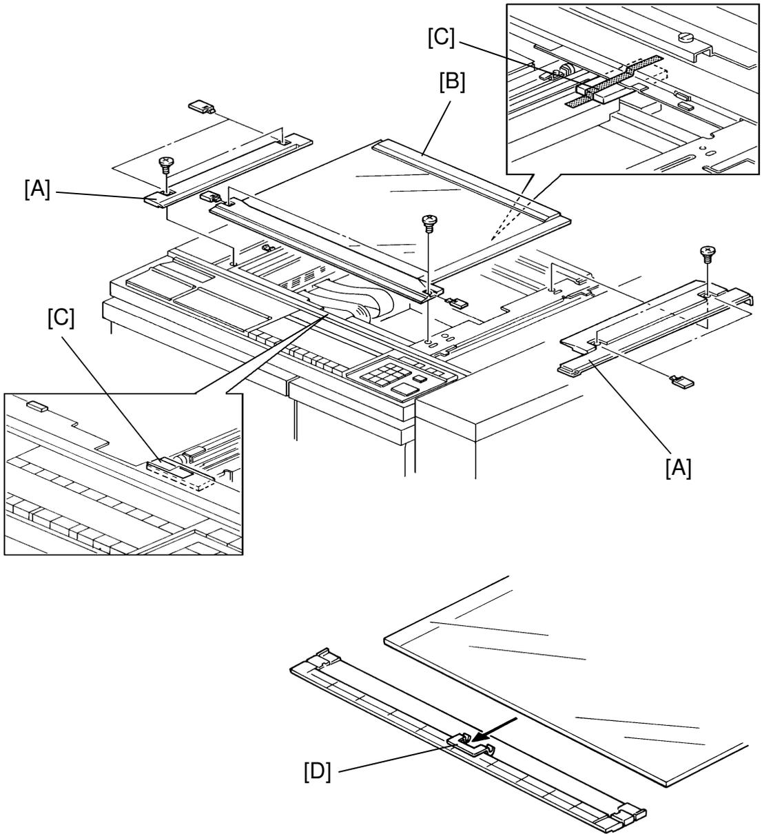
15. Remove the right and left scales[A] (2 screws each), remove the front scale (2 screws) with the exposure glass [B]. Be careful not to lose the plastic screw covers.
