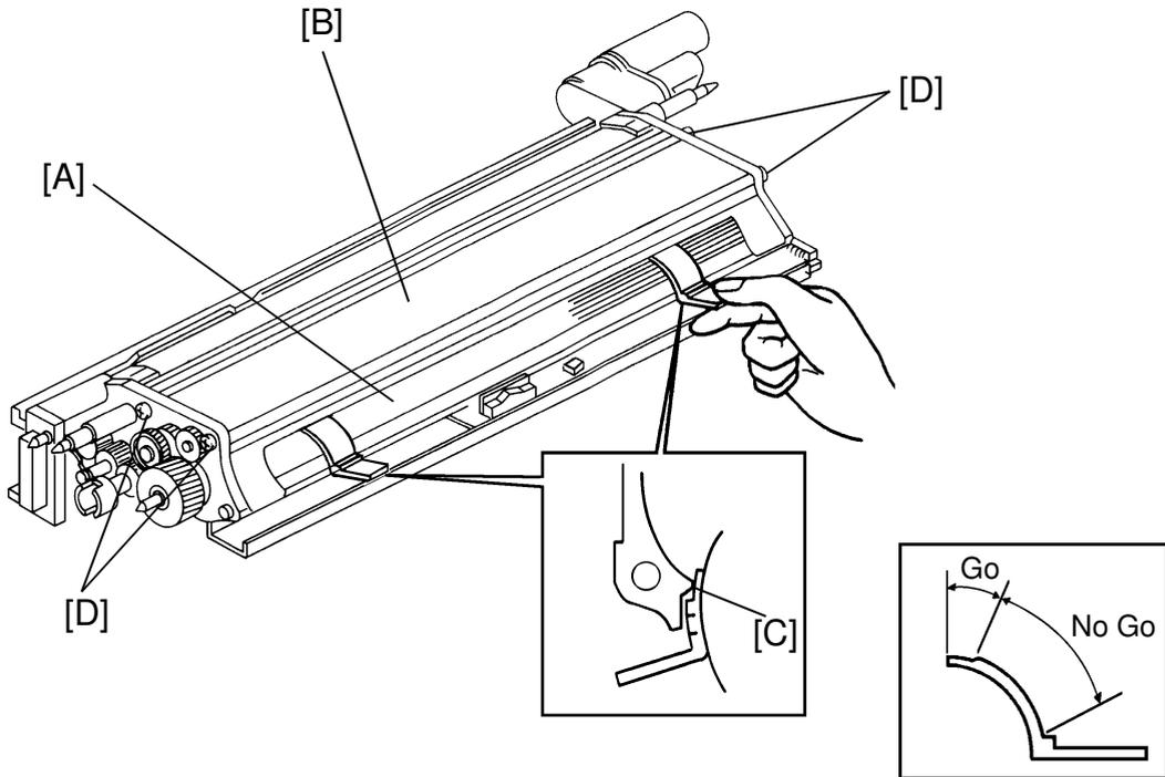
1. Clean the development roller [A] with a vacuum cleaner until no developer is on the roller. Turn the roller to make sure that it is free of developer.
