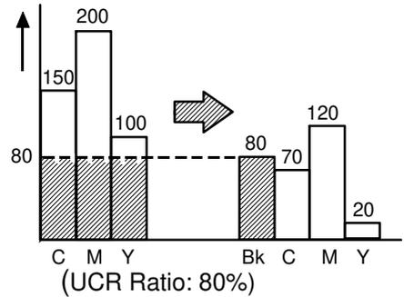
The black output is determined by the CMY data (which is a result of the RGB data). A common value is subtracted from the C, M, and Y values and this value becomes the black value. This is called UCR (Under Color Removal).
