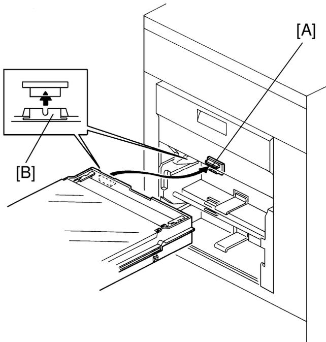
An array of five photointerruptors [A] in the cassette entrance detects the paper size. The paper size sensors are actuated by a plate [B] on the front of the cassette. Each paper size has its own unique combination of notches in the actuator plate. The CPU reads which photointerruptors have been blocked de-actuated by the actuator plate to determine which paper size has been inserted.
