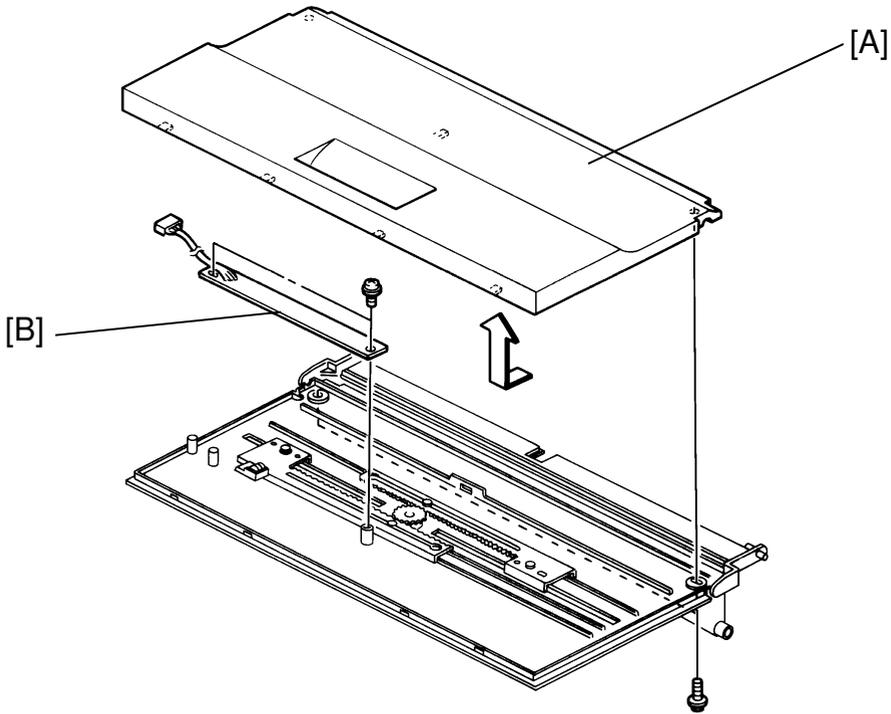
1. Remove the by-pass feed table (see By-pass Feed Table Replacement).
