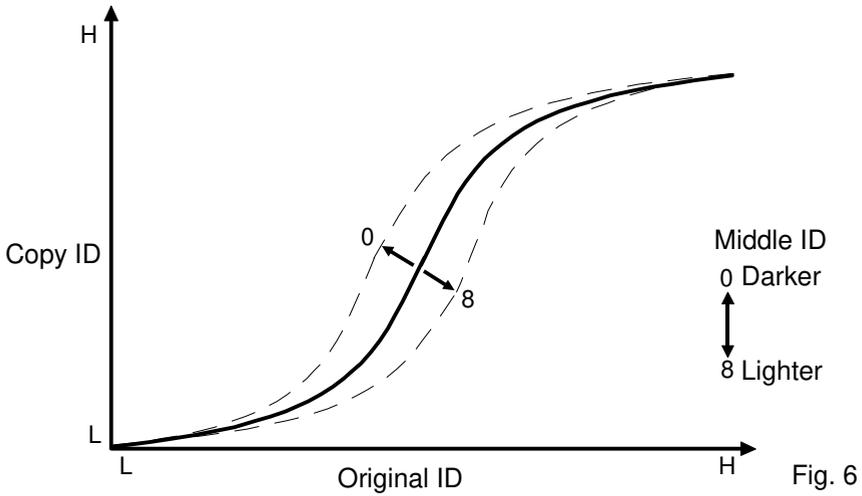
Middle ID is used to adjust the image density for all ID levels (figure 6).
