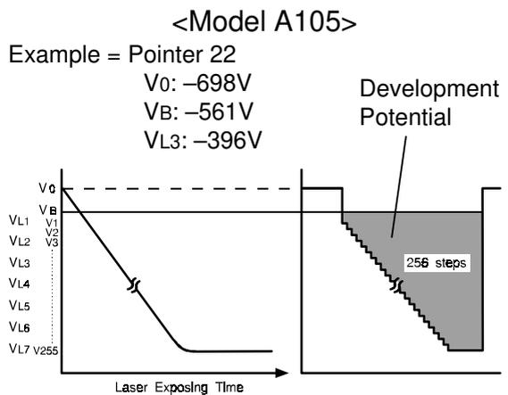
Most copiers use either a positively charged photoconductor and negatively charged toner or a negatively charged photoconductor and positively charged toner. This is known as positive/negative development. However, this machine uses a negative/negative process where both the drum surface charge and the toner charge are negative.
