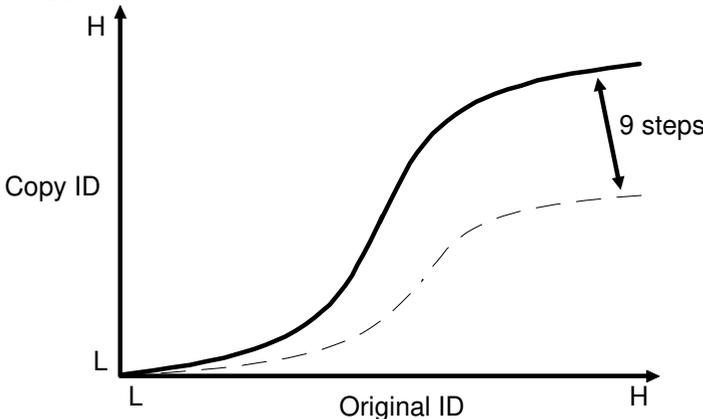
This function can be used to decrease the copy density more than by using image density control. The image will become pastel.
