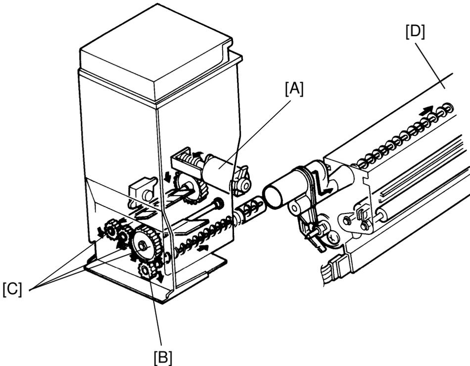
When the toner supply motor [A] turns on, two agitators begin rotating clockwise to agitate the toner inside. The rotation of the toner supply motor is also transmitted to the transport coil gear [B] through the agitator gears [C] and the toner is then transported to the development unit [D].
