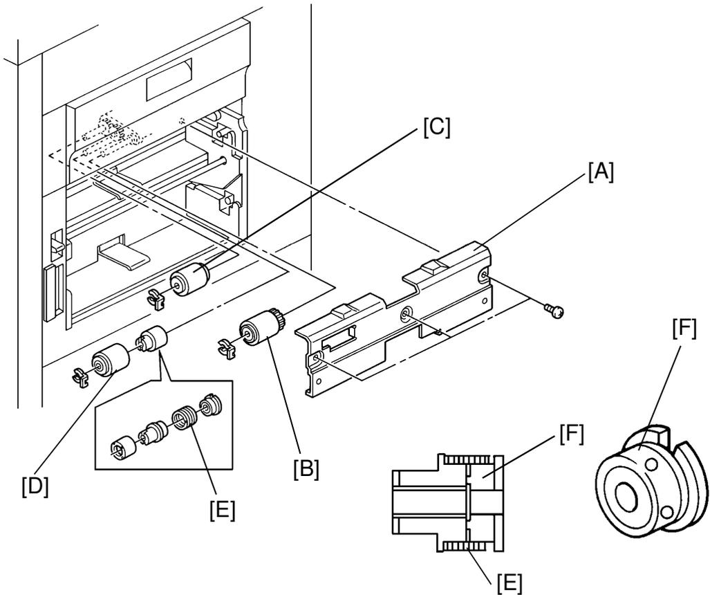
1. Remove the cassette and the feed-in roller cover [A] (3 screws).
