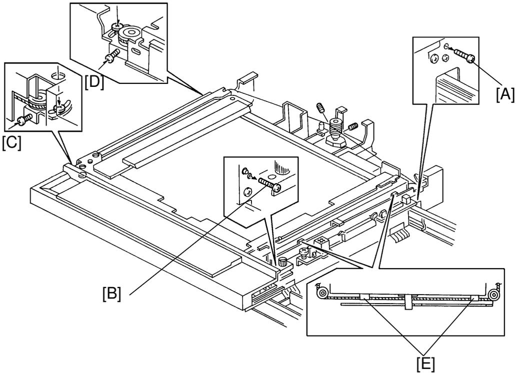
11. Loosen the Allen screw. Take the scanner motor pulley from the temporary support, and place it on the scanner motor shaft.
