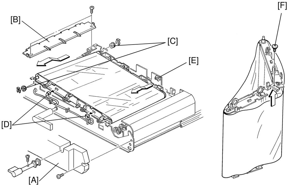
1. Turn the transfer unit stopper lever counter-clockwise using a minus screwdriver to pull the unit all the way out.
