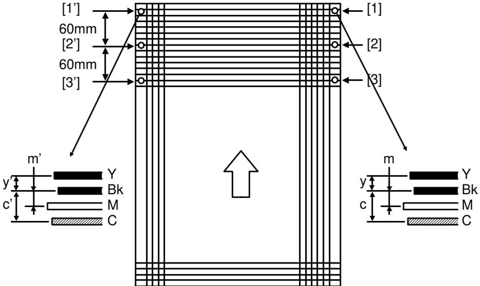
1. At point [1], measure the distance between each color line and the black line (y, m, and c) as shown in the illustration.
