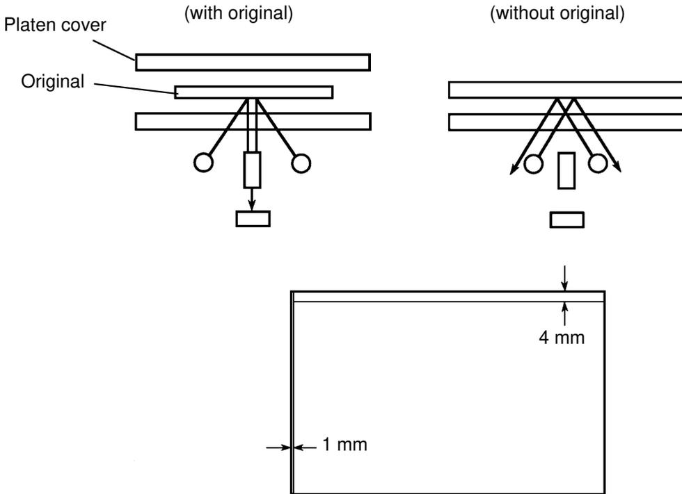
When the original is scanned, the light from the exposure lamps is reflected and the image is sent to the CCD board by diffuse reflection. Since the platen cover sheet of this copier acts like a mirror, at the non-original area, the light cannot reach the CCD board because of the spicular (mirror-like) reflection. By using the difference in reflected light intensity, the original size is determined.
