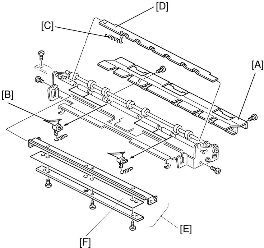
1. Remove the cleaning roller (see 12.11 CLEANING ROLLER REPLACEMENT).
