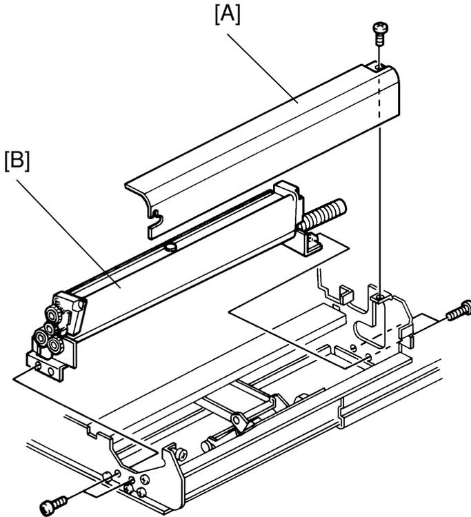
1. Remove the transfer unit (see Transfer Unit Removal).
