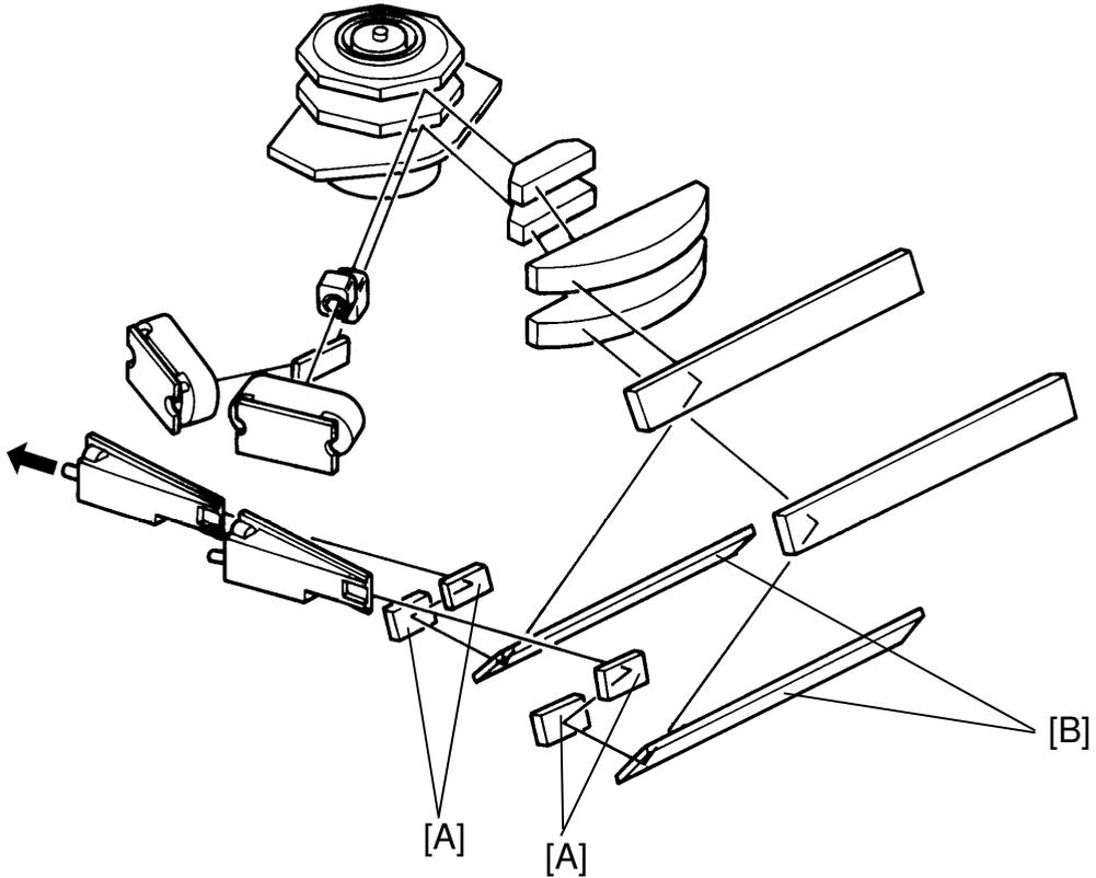
At the start of each scan line, the synchronizing mirrors [A] and the 2nd drum mirrors [B] reflect the laser beam to the laser synchronizing detector, as shown above.
