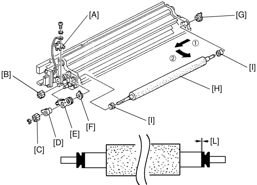
5. Remove the grounding bracket [A] (1 screw, 1 star washer). Remove the gear [B] (1 E-ring), the gear [C], the bushing [D], the bracket [E] and the bushings [F] [G] in order.
