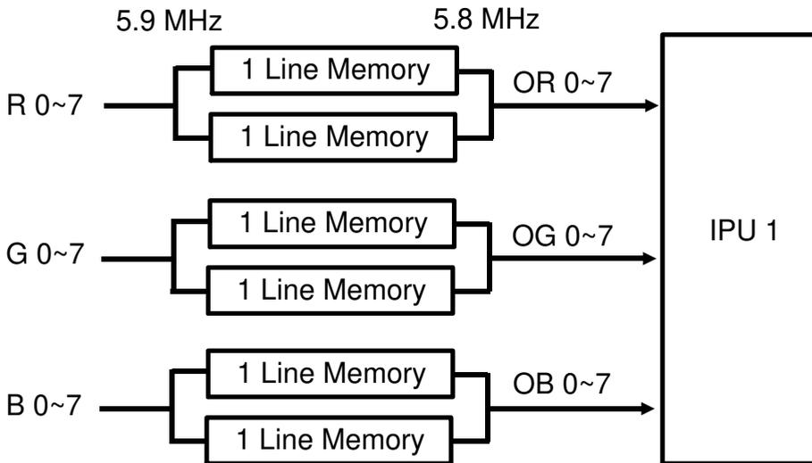
The clock frequency of the scanner control board is 5.9 MHz. The clock frequency of the IPU1 is 5.8 MHz. To meet the data transfer timing, 1 line memories are adequate. There are two 1 line memories for each color. When scanning the original, one line video data is stored in the 1 line memory. This data is transferred to IPU 1 when next line data is stored in the other 1 line memory. Therefore, 1 line memory is a kind of buffer and it can adjust the output rate.
