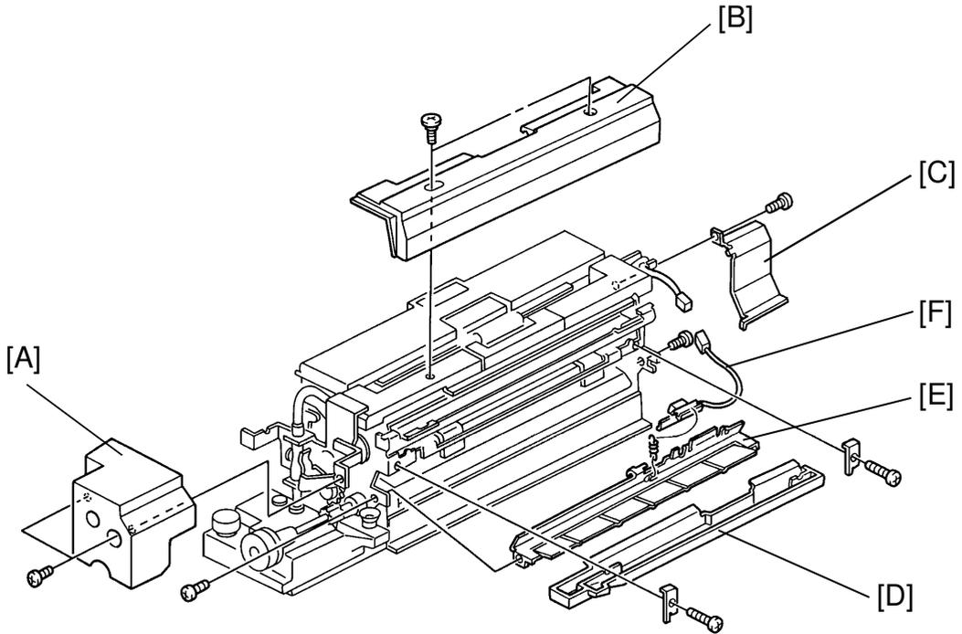
1. Remove the cover [A] (two M4 x 8 screws).
