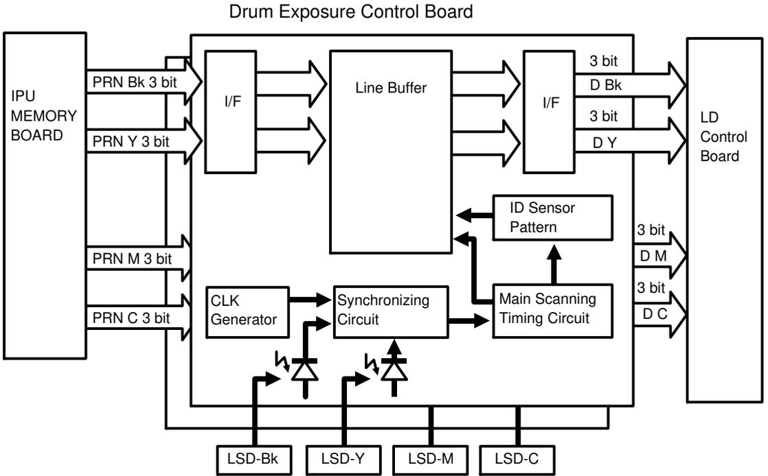
Two drum exposure control boards are used in this machine. One is for black and yellow laser exposure and the other one is for magenta and cyan laser exposure. These boards have the following functions:
