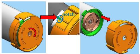
20\*. Install the new toner cartridge[A]. (You can refer to the decal attached to the left side of the machine.)
