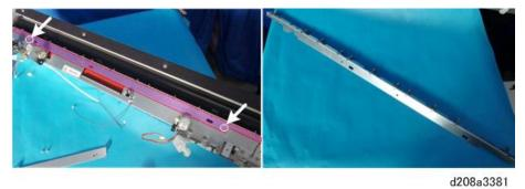
7. Remove the pressure roller [1] from the fusing unit.
