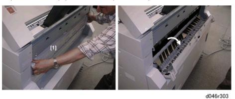
2. Grip the rings on both ends of the paper exit guide [1], pull it toward you to release it, and lower the guide.
