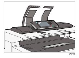
The original stackers can hold one original at a time. Remove each original by holding its leading edge after it is ejected.
