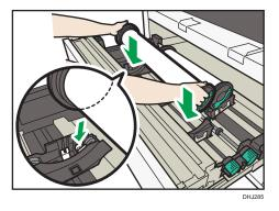
Make sure that both ends of the paper holder are securely seated in the grooves of the roll holder.
