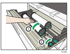
5. Keep pressing the auto feed button until the edge of the paper emerges from the cutter section (①), and then remove the cut piece of paper (②).
