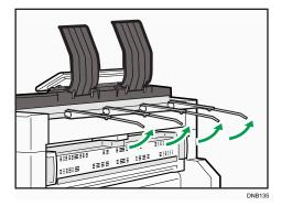
Originals are ejected onto the original output guides.
