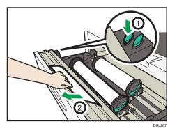
The paper will be cut automatically when you release the feed button.
