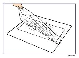
2. Using both hands, hold the carrier sheet face down, and carefully insert the folded edge of the carrier sheet into the insertion area.
