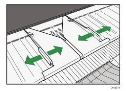
2. Using both hands, carefully insert the original between the original guides, copy side down.
