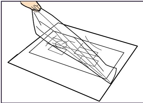
2. Using both hands, hold the carrier sheet face down, and carefully insert the folded edge of the carrier sheet into the insertion area.
