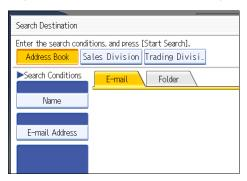
If authentication is required to access the selected server, the authentication screen appears. To authenticate, enter the user name and password.
