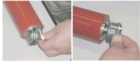
5. Remove the pressure roller [1] from the fusing unit.
