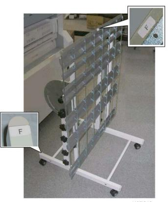
1. Make sure that the "F" mark on the stacker tray is on the same side as the "F" marks on the legs.
