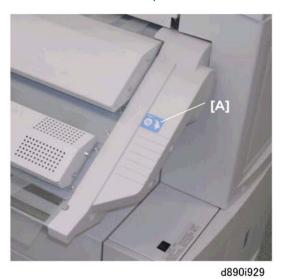
3. Attach "N1" decal [A] to the right side cover of the bridge unit.
