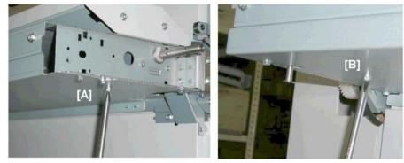
8. Fasten shoulder screws to the paper entrance unit on the left end [A] and right end [B] ( $\hat{\mathscr{F}}$  x2).
