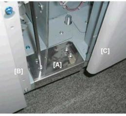
9. Attach the rear brace [A] between the transport unit [B] and cross fold unit [C] ( $\hat{\mathscr{F}}$  x4 M3x8).
