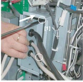
9. Reattach the inner cover [1] to the rear of the main machine ( $\hat{\mathscr{F}}x2$ ).
