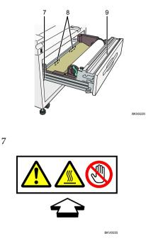
The inside of the machine could be very hot. Do not touch the parts which a label is put on. Otherwise, an injury might occur.
