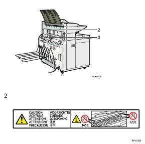
Do not touch the parts a label indicates. The inside of the machine could be very hot. Caution should be taken when removing misfed paper. The higher temperature (145°C) applies to plain paper. Translucent paper can cause the indicated part to reach 160°C.
