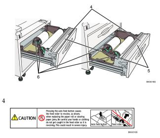
Pressing the auto feed button causes the feed roller to revolve, as shown, when replacing the paper roll or clearing paper jams. Be careful your hands or clothing do not get caught in the feed roller as it is revolving. This could result in severe injury.
