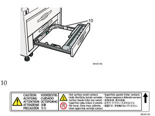
The inside of the machine could be very hot. Do not touch the parts a label indicates. Otherwise, an injury might occur.
