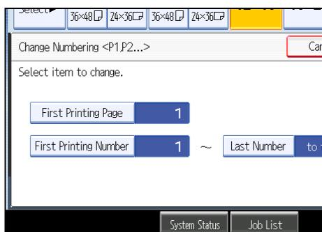
6. Press [First Printing Number], enter the number of page from which to start numbering with the number keys, and then press [#].
