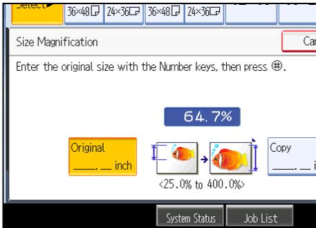
You can enter sizes between 1 to 9999 mm (0.1 to 99.9 inches) in increments of 1 mm (0.1 inch).
