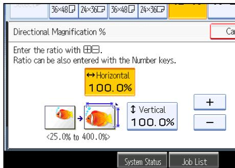
Pressing [+] or [-] changes the ratio in increments of 0.1%. Pressing and holding down [+] or [-] changes it in increments of 1%.
