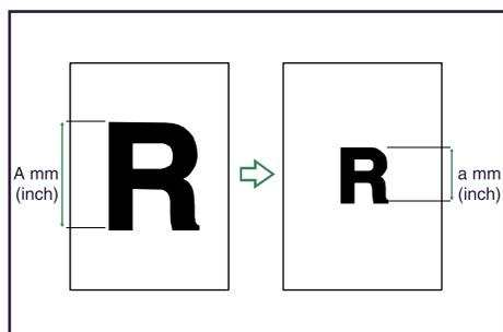
Measure and specify the lengths of the original and copy by comparing "A" with "a".
