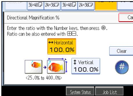
4. Enter the desired ratio with the number keys, and then press [#].
