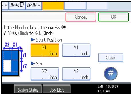
5. Enter the lengths of [X2], [Y1], and [Y2] in the same way, and then press [OK].
