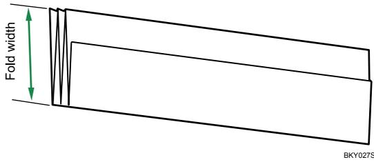
If the Fan Folding Finisher is installed, you can select a fold width of 140, 170, 210, or 297 mm (8<sup>1</sup>/<sub>2</sub>", 9", 11", or 12"). When [210mm(Margin Fold)] is selected, paper is folded so as to have a binding margin. If the Cross Folding Finisher is installed, you can select a fold width of 140, 170, or 210 mm (8<sup>1</sup>/<sub>2</sub>", 9", or 11").
