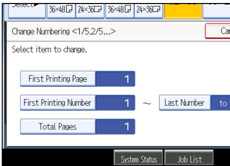
6. Press [First Printing Number], enter the number of page from which to start numbering with the number keys, and then press [#].
