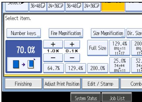
Press [+] or [-] changes the ratio in increments of 0.1%. Pressing and holding down [+] or [-] changes it in increments of 1%.
