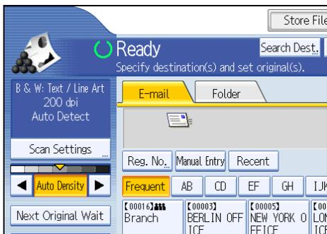
**2. Using the number keys, enter the five-digit registration number assigned to the required destination.**
