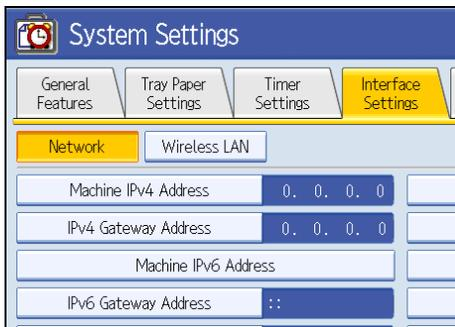
3. Press [Machine IPv4 Address] to specify the machine's IPv4 address.
