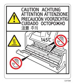
The inside of the machine could be very hot. Do not touch the parts a label indicates. Otherwise, an injury might occur.
