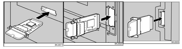
Insert the end of the wireless LAN interface unit into the slot.
