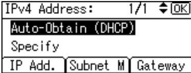
The printer will automatically receive an IP address.
