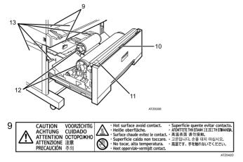
The inside of the machine could be very hot. Do not touch the parts which a label is put on. Otherwise, an injury might occur.
