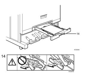
When replacing or loading the paper, or clearing paper jams, pull out the cut paper tray slowly with both hands. Do not pull out the cut paper tray with a single hand. Otherwise the rear of the cut paper tray may fall and an injury may result.
