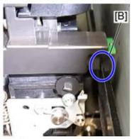
A transparent sheet is attached to the service part of the horizontal encoder sheet for protecting the part. Peel off the protective sheet before attaching the part.
