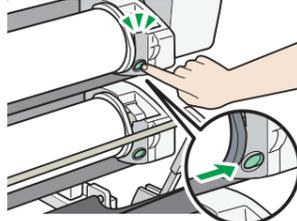
After you release the button, the paper is rewound automatically. If the paper is not rewound, press the button again. If there is no paper roll loaded, proceed to Step 4 of "Inserting the Spool into the Paper Roll".
