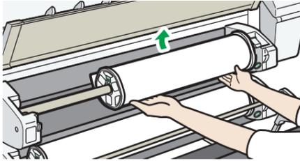
When you insert the paper between the guides, it is clamped and pulled into the machine.
