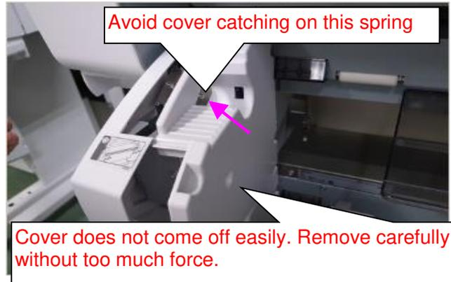
6. Remove the support bracket. (screw x4)
