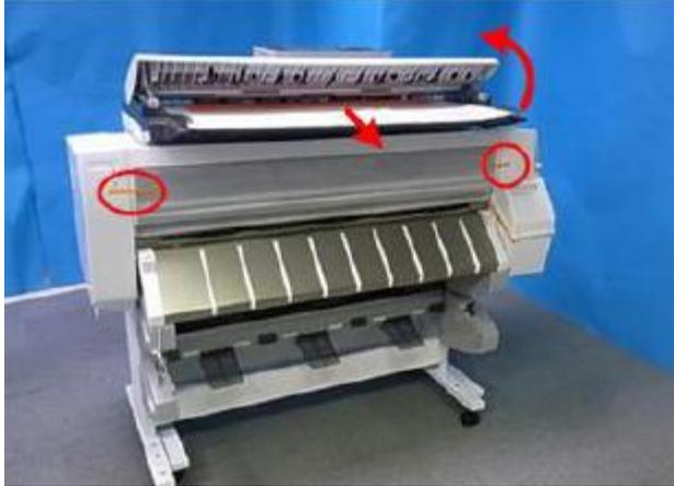
3. Lift the front cover, and then fold the bottom into the machine so that it locks and remains open.
