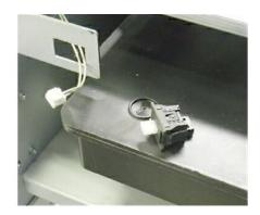
3. Pull the switch through the frame and disconnect it ( $\mathfrak{C}$  x1).
