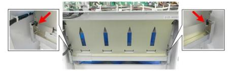
5. At the bottom of the guide plate, make sure that the left and right corners are seated correctly.
