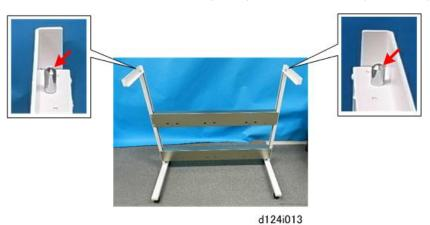
1. Locate the vertical positioning pins on top of both sides of the assembled scanner stand.
