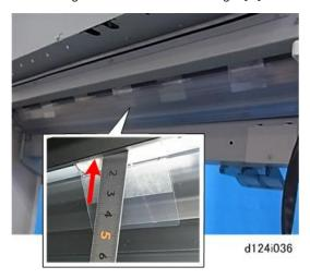
14. Use a thin edge (like the end of a metal scale) to push the tongues of the guide mylar up and behind the plate. There are six mylar tongues.
