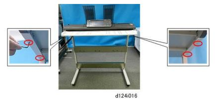
6. Set the scanner unit down on the positioning pins, then fasten the unit to the stand ( $\checkmark$  x4 - M4x8).
