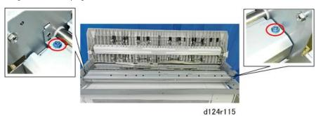
1. Disconnect the left and right ends of the original width sensor cover plate (  $\nearrow$  x2).
