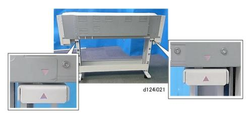
5. Position the main unit over the top of the stand so that the triangle marks at the rear are aligned (X).
