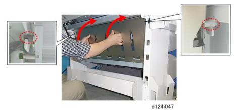
19. Behind the machine, hold the guide plate as shown, and then set the cut-outs on the left and right over the pegs.
