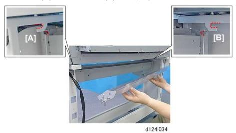
11. While holding the paper transport guide with both hands as shown above, insert the pegs on either end of the guide into the cut-outs in the stand on the left [A] and right [B]. The guide should slide into position and fit snugly after correct alignment.
