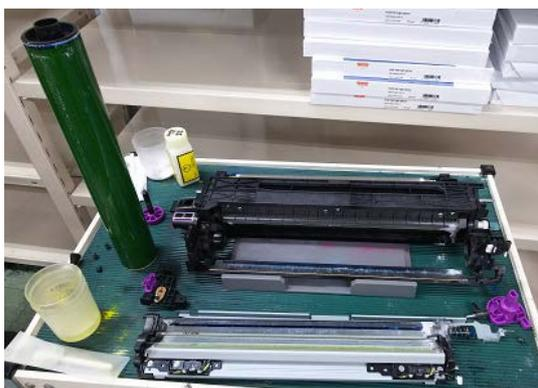
7. Using the blower brush (D0747690), clean the drum, toner catcher of the development unit, and toner receptacle at the bottom of the drum cleaning unit. Then, apply the lubricant powder (D0159501; zinc stearate) across the entire surface of the drum evenly.
