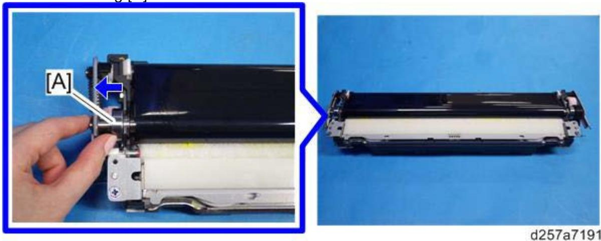
5. Remove the two screws, and then rotate the bracket [A] in the direction of the blue arrow.
