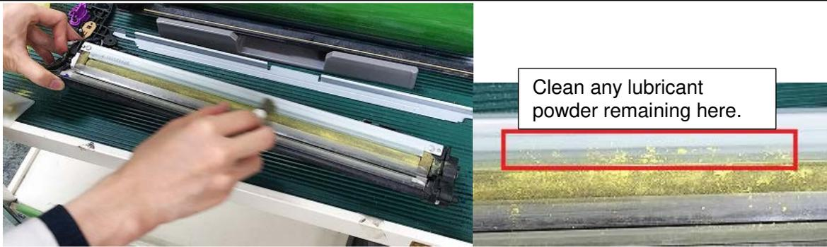
**When the drum cleaning unit was not replaced**
