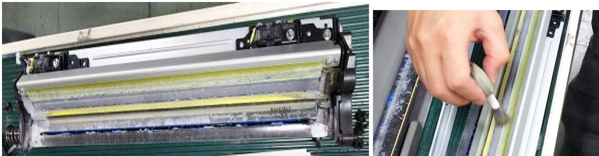
NOTE: Do not use a vacuum cleaner. Clean the cleaning blade with the blower brush until you confirm no lubricant remaining on the cleaning blade. To drop waste toner to the toner collection coil, tap the casing at the opposite side of the cleaning unit. Clean the entrance seal positioned toward the lubricant blade. Do not rotate the lubricant roller, to prevent the lubricant powder from dropping. Clean any dust observed.
