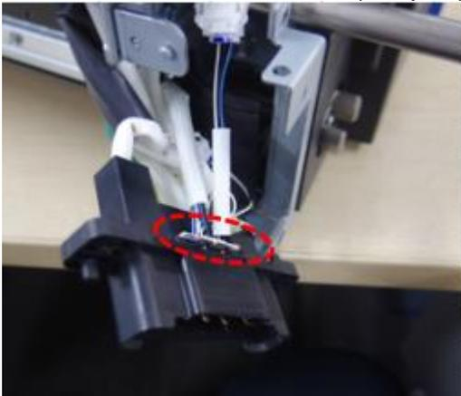
5. Remove the relay connector holder (1 screw).
