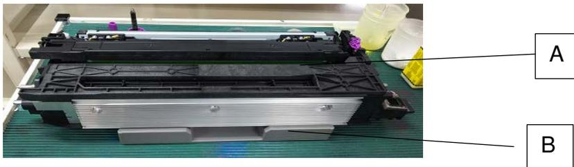
3. Remove the charge roller unit [A].
