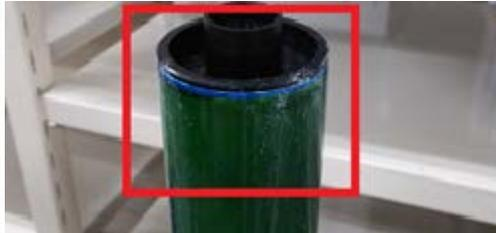
NOTE: Heavy load is put on the edges of the drum. Make sure to apply the lubricant powder at both edges evenly.
