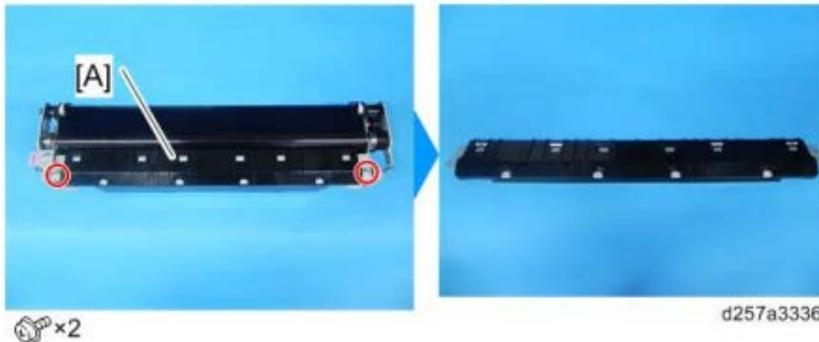
3. Remove the pressure springs [A].
