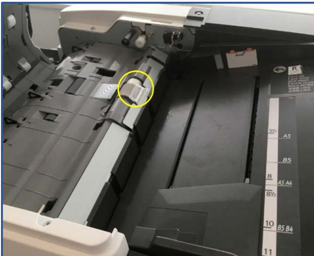
3. Remove the paper feed guide plate.
