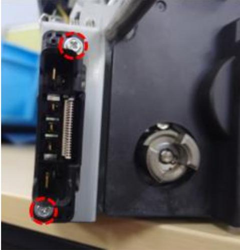
4. Remove the DC connector (snap fit).
