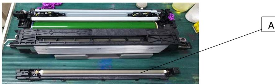
**NOTE:** After removing the charge roller unit, place it on a clean, flat surface with the roller facing up.
