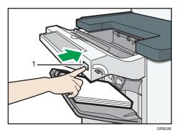
1. Press the [Suspend / Resume] key near the paper outlet port.
