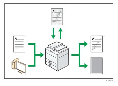
Using the copier function or the printer driver, you can embed a pattern in the printed document. If
