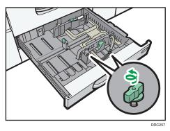
5. While pressing down the release lever of the side fence, slide the side fences outward.
