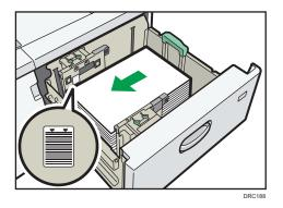
10. While pressing the release button of the end fence, align the end fence gently against the paper you loaded.
