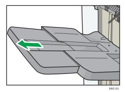
4. Attach the thin paper support tray by setting its protrusions onto the back fence of the finisher shift tray.
