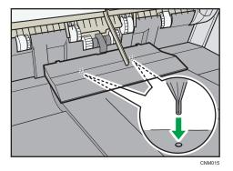
Attach the Z-fold support tray 3 by inserting the two protrusions on its underside into the holes on the finisher shift tray.
