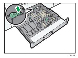
4. Loosen the screws holding the side fences in position.
