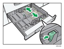
6. While pinching the release lever of the end fence, slide the end fence outward.
