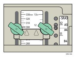
8. Hold the inner side fence, and then tighten the screws to the inner side fence.
