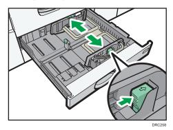
6. While pinching the release lever of the end fence, slide the end fence outward.
