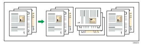
To use the Rotate Sort function, two paper trays loaded with paper of the same size and type, but in different orientation ( $\square \square$ ), are required.
