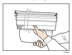
2. Holding its shorter ends, flex the stack back and forth to create space between the sheets. Repeat this several times.
