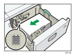
10. While pressing the release button of the end fence, align the end fence gently against the paper you loaded.
