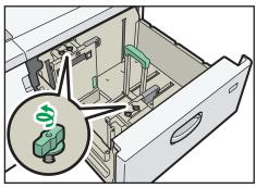
4. Hold the indents at the bottom of the side fences with your fingers, and then slide the side fences outward.
