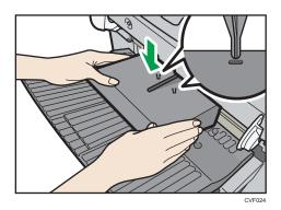
Attach the Z-fold support tray by inserting the two protrusions on its underside into the holes on the finisher shift tray.
