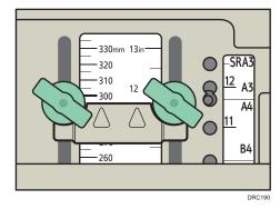
8. Hold the inner side fence, and then tighten the screws to the inner side fence.
