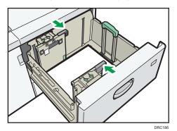
Check that the positions of the scale numbers on the top of both of the side fences are almost the same. When loading regular size paper, align the screw holes on the side fences to the paper size mark.
