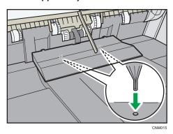
Attach the Z-fold support tray 3 by inserting the two protrusions on its underside into the holes on the finisher shift tray.
