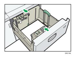
Check that the positions of the scale numbers on the top of both of the side fences are almost the same. When loading regular size paper, align the screw holes on the side fences to the paper size mark.
