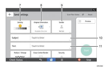
No. Icon Description Press to specify the density to scan the original. 7 You can also specify the density by touching the 🔔 icon and dragging it right or left. €R Press to select the orientation of the original. 8 Press to specify the sender. 3 9 10 Subject Press to enter the subject of the e-mail. Text Press to enter the main text of the e-mail. 11
