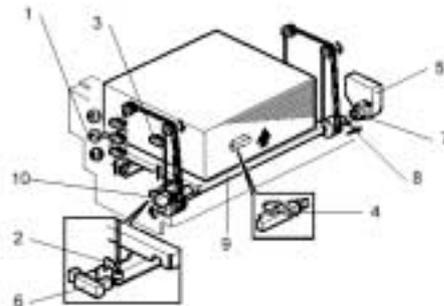
**Paper remaining:** The amount of paper remaining in the tray is detected by which combination of the three paper height sensors [1] ❶, ❷, ❸ are actuated by the actuator on the left rail as the bottom plate rises.
