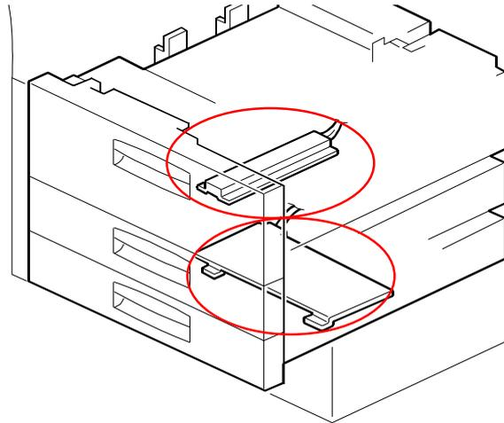
**These two heaters must be connected during the installation procedure for the copier, if the customer wants to use them.**
