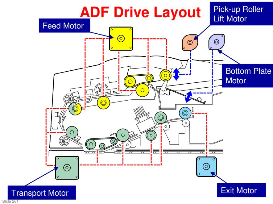
**Pick-up roller lift motor: Drives the pick-up roller lift mechanism.**
