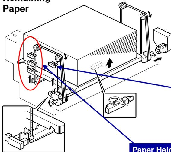
❑ Paper height and near-end sensors: Detect amount of paper remaining
