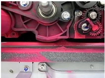
6. Gap between charge roller and drum
