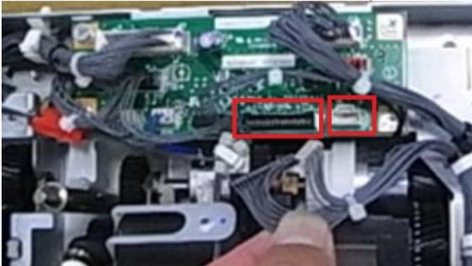
4. Remove the clamps (x3) and hang the free end of the harness over the hopper duct, as shown.
