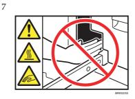
Do not touch the parts a label indicates. The inside of the machine could be very hot. Caution should be taken when removing misfed paper.
