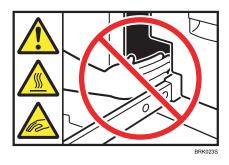
Do not touch the parts a label indicates. The inside of the machine could be very hot. Caution should be taken when removing misfed paper.
