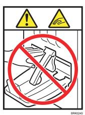
Do not touch the paper exit section of the finisher. It could cause injury.
