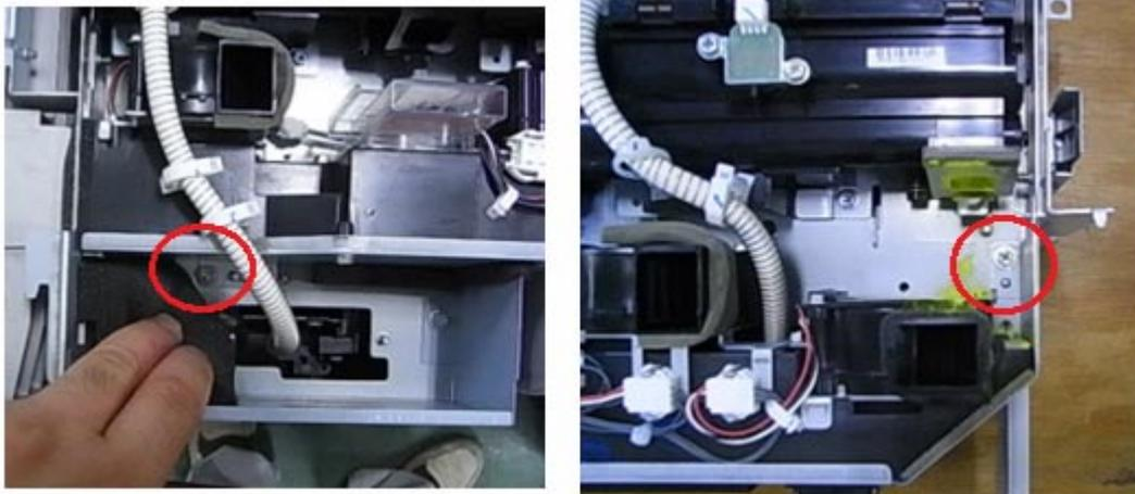
6. Remove the toner supply tube from the black toner supply unit (🔩 x3).
