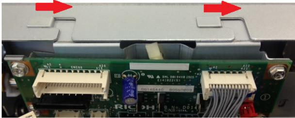
7. Remove the bracket, rotate it upside down and to the right, and then place it on the sheet of paper as shown.
