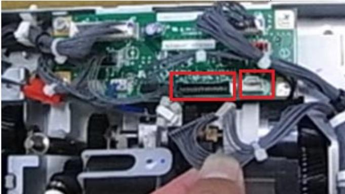
4. Remove the clamps (x3) and hang the free end of the harness over the hopper duct, as shown.
