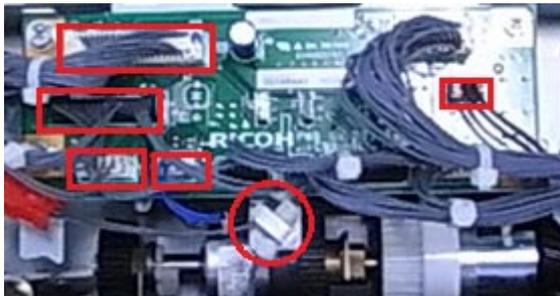
4. Remove the screw (x1) from the CNB board bracket.
